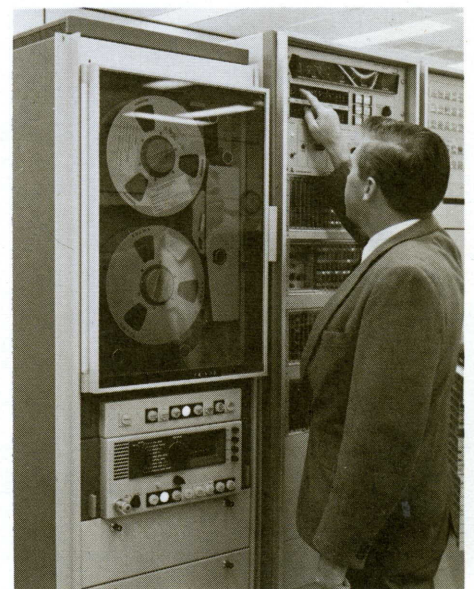
Gerald G. Leeson prepares to reproduce a tape on an Ampex FR-900 at NASA Houston containing pictures from the Lunar Orbiter I Moon shot. Leeson, Acting Supervisor, Lunar Orbiter Data Conversion System, is with Lockheed, a support contractor for NASA.
