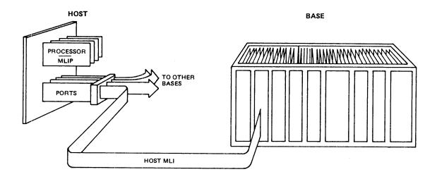
Each I/O base contains one or more Data Link Processors (DLPs), which function as peripheral controllers. PT-DLP handles both the printer and the tape drive; disks have different DLPs, depending on the type of disk used. Network Support Processors (NSPs) and Line Support Processors (LSPs) are programmable DLPs that provide data communications services. A DLP can be connected to a peripheral directly, to a peripheral controller, or, if an NSP, to another base.
