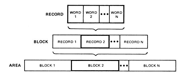
It can be helpful to a site to standardize the size of all areas to 504 sectors, the area size of object files produced by the compilers. This can help prevent "checkerboarding" of the disk, where available disk space is fragmented into areas too small for the file areas.
