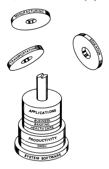
The first or foundation layer performs overall system control and so-called "housekeeping" functions, and is known as system software. This software consists of the operating system, which can be either the Master Control Program/Advanced Systems (MCP/AS) or the Master Control Program (MCP), the system utilities, and the language compilers.
