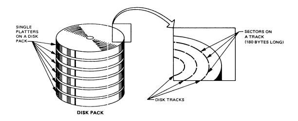
Data is written to and read from disk volumes on a disk drive that has one or more read/write heads. These heads are positioned over the desired tracks of the spinning disk so that information can be stored and retrieved from those tracks.
