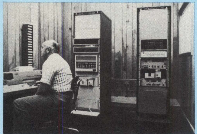
Fig 1 Hewlett-Packard 9600 automatic measurement system at load dispatch center of U.S. Steel's Geneva Works in Utah. For past four years system has monitored conditions of motor and generator bearings as well as operation of water recycler and has calculated natural gas usage within daily allocations. Capacity remains for enhancement to handle other duties still in planning stages
