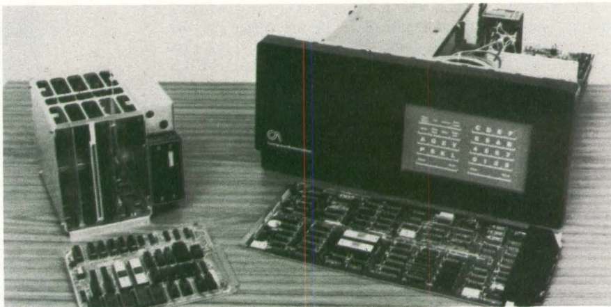
Processor board of Computer Automation's Scout 4/04 (left foreground) is about half the size of LSI 4/10's CPU board. Overall size reduction is dramatic when power supply, chassis, and memory and logic boards are included in comparison
