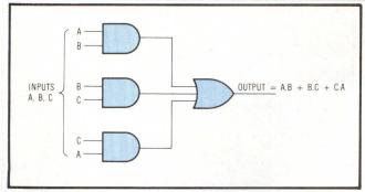
Fig 2 Simplified hardware voting scheme to achieve fault tolerant data. Such a scheme does not prevent faults internal to voting circuit from producing errors.
