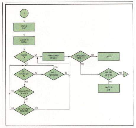
Fig 5 Prime field service systems procedures are a continuation of manufacturing qualification program and provide further data on new chips based on actual customer site operation.
