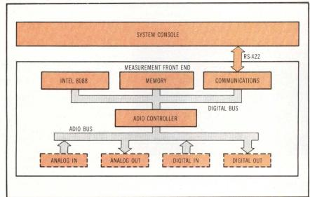
Block diagram of Macsym 350 measurement and control system. Library of 32 different I/O cards is available for attachment to ADIO bus.
