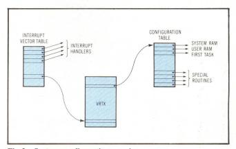
Fig 2 System configuration requires programmer to supply only one address that connects operating system to application. User supplies configuration table.
