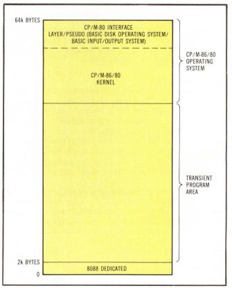
Fig 2 Shared RAM memory map. 62k-byte shared area provides space for the CP/M operating system as well as applications programs.
