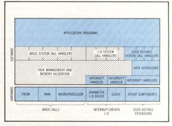
Fig 1 Typical component operating system structure. Dashed areas indicate functions provided by system nucleus. Only hardware assumptions made are specific microprocessor being used, and existence of 1k of RAM.
