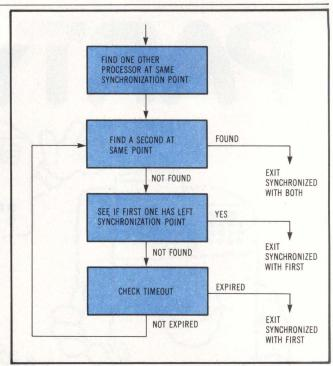
Fig 6 Synchronization tests protect against malicious fault occurrence.
