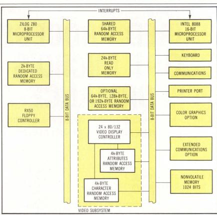
Fig 1 Dual-processor architecture. Each microprocessor unit employs dedicated and shared resources for more efficient use of hardware while maintaining software compatibility.
