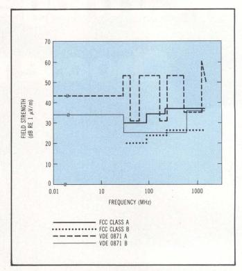
Fig 4 Comparison of FCC and VDE radiation emission limits for Class A (commercial) computer equipment. FCC is stricter in the 30-MHz to 1000-MHz region.
