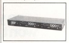
IFA-18 current loop adapter furnishes conversion between 20/60-mA current loop and RS-232/V.24 environments. Adapter provides electrical and mechanical compatibility for differences between current loop and RS-232 equipment. Monitor channel can be used with std RS-232/V.24 data monitors and is compatible with the company's line of interface converters. Unit can be mounted desktop or in a 19" (48-cm) rack assembly. Atlantic Research Corp, 5390 Cherokee Ave, Alexandria, VA 22314. Circle 293
