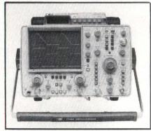
1746A 100-MHz oscilloscope with large screen CRT and dual-marker time interval measurement system. Optional DMM provides measurements of ac/dc voltage, ac/dc current, and resistance. DMM improves accuracy of time interval measurements.
