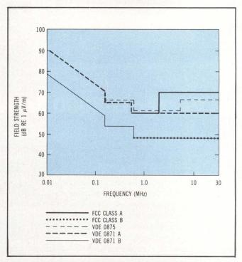
Fig 5 Comparison of FCC and VDE conducted emission limits for Class A (commercial) hardware. VDE 0871A and B curves, from 150 kHz to 10 kHz, represent proposed limits. Note that some requirement levels overlap.
