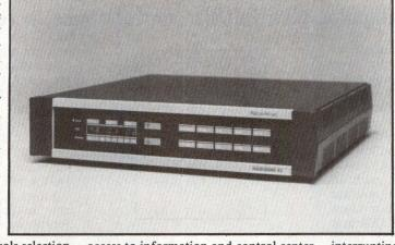
The front panel also controls selection and change of modem speed, port configuration, transmit level, strapping, modulation, and training method. The panel locks against unauthorized use or data interruption and allows authorized use via password entry. Firmware based for flexibility, the modem can operate in domestic data networks when software strapped as an MPS 48 or as an MPS 4827 for international CCITT V.27 compatible applications. Internal hardware straps are eliminated
