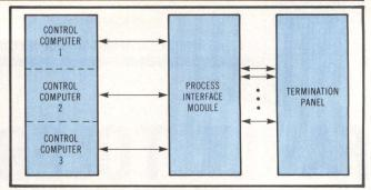
Fig 1 Fault tolerant computer architecture of August 300 system. Three computers analyze each other's results via read only data link.
