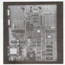
modules for analog signal conditioning, A-D conversion, and digital I/O. An onboard STD BUS connector allows use of previously designed and custom STD BUS functions. In small volumes and during application development, the modules are in plug-in card format and use Eurocard connectors. In production quantity,
