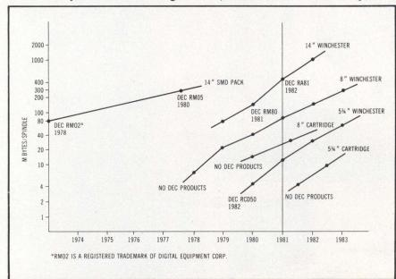
Mass storage capacity advances for typical large mainframe manufacturer. Extended integration cycles and inadequacy of evolved operating systems keep large computer makers one to four years behind mass storage state of the art.
