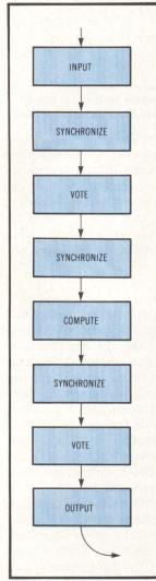
Fig 4 Control program flow incorporating processor synchronization. Periodic rendezvous of redundant elements eliminates errors due to timing or sampling discrepancies.
