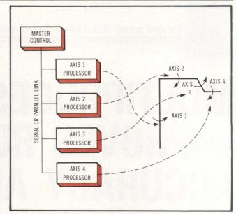
Fig 2 Multiprocessor robotic system with processor for each axis. Master processor supplies angular position and time frame, as well as loading and stress factor information to adjust algorithm for maximum accuracy.
