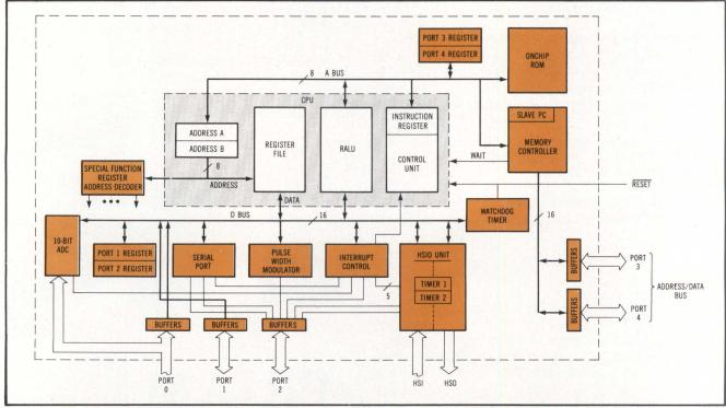
Simplified block diagram of 8396 16-bit microcontroller. Memory to memory architecture is organized around dual buses. Five 8-bit I/O ports include input only (port 0), quasi-bidirectional I/O (port 1), multifunction (port 2), and two bidirectional (3 and 4).
