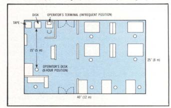
Fig 3 Physical layout of office/design space used in calculations and measurements of acoustic levels
