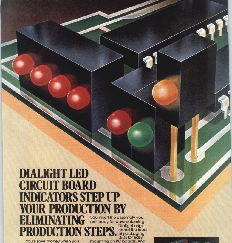
You'll save money when you stop mounting LEDs on PC boards the old way — bending leads, inserting holders, adding resistors — and start using LED Circuit Board Indicators from Dialight.
