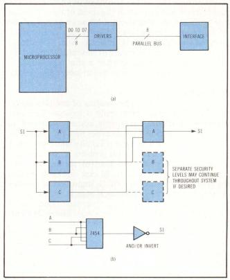
Fig 5 Typical digital system interconnect. Eight-bit parallel data bus of (a) is protected from failure by triplication of signal paths (b). Inevitable increases in wire reduce reliability and foster noise and crosstalk problems.
