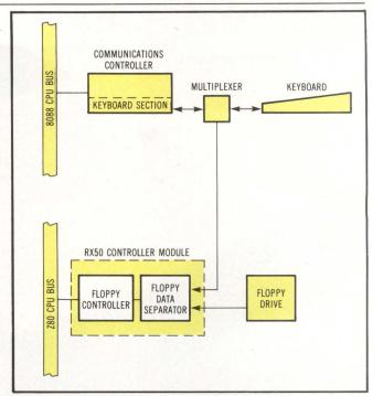
Fig 4 Internal loopback testing of system components is possible. Failures may be pinpointed beyond peripheral level to system components. Here floppy controller, data separator, and system board are checked.
