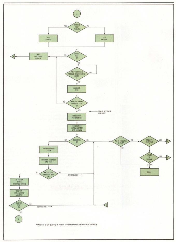
Fig 4 Prime's manufacturing qualification of 64k DRAMs. Here, more rigorous tests are run on the same devices, both individually and in product environment, before production procurement is approved.
