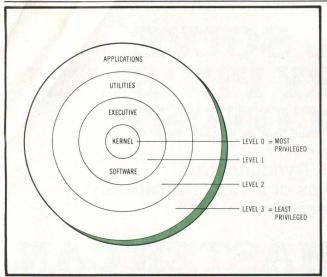
Fig 3 Privilege levels available in iAPX 286 protection model. Note use of small kernel to eliminate excessive operating system access of data base.
