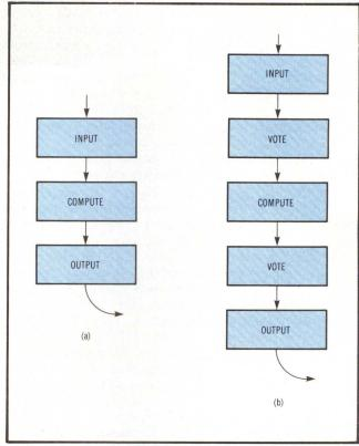
Fig 3 Typical control program sample loop in (a) can be modified to perform voting operation associated with fault tolerance (b).
