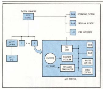
Fig 1 Single-board robot control unit. Six-layer PCB performs 10 MIPS and features six 6800-type axis processors running under control of one 68000 processor.
