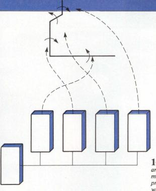
169 A master processor supplies angle, loading, and stress data to individual axis processors in a multi-axis robotic system. Both master and axis processors are powerful single-chip microcomputers with large amounts of onchip 1/0.
