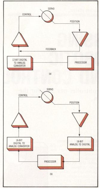
Fig 1 Typical robotic control loop yields positional accuracy of 0.05" (0.13 cm) (a). Digital control loop improves accuracy to 0.02" (0.05 cm) or better (b).
