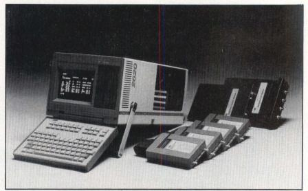
Field maintenance processor 2620. Plug-in architecture features patented device specific adapter bus and four adapter slots to provide capability for universal product interface. Special function keys allow single keystroke initiation of lengthy test sequences or test mode specification.
