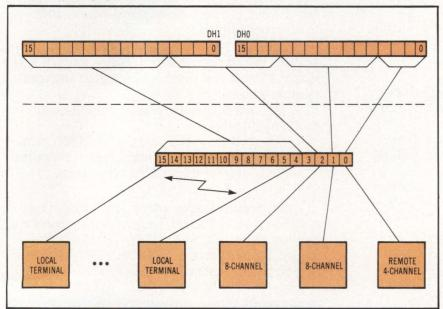
Remote terminal clusters can be allocated channels from separate DH11 interfaces. This is also true of 8-channel DZ11 interfaces. Note that port 3 remains unused after local and remote terminals are allocated all 32 channels.
