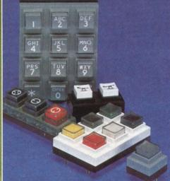
SERIES 83-84-86 Short stroke standard 3x4 and 4x4 keyboard configurations. Choice of ½ inch or ¾ inch button centers and post or flange mounting. Standard coded outputs—easily interfaces with logic circuitry. Excellent audible and tactile feedback.
