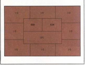
Fig 4 Alterable microcomputer functional block diagram. Core processor is integrated with required amounts of RAM and ROM, together with library cell or fully customized 1/O and peripheral functional modules.
