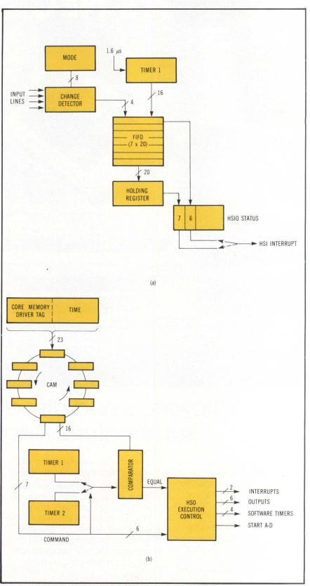
Functional diagrams of 8096/8396 HSI and HSO units. HSI unit (a) sees input line transitions and stores input line number and transition time in 8-deep FIFO. Unit can be programmed to activate HSI data available interrupt. HSO unit (b) can be programmed to cause output line transitions.
