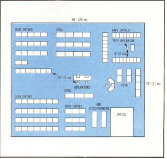
Fig 1 Physical layout that serves as basis of mathematical model of medium to large DP center used to determine acoustic measurements
