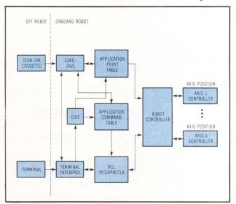
Fig 3 Software architecture overview. Segmented software supports six axis controllers in real time and supplies system and housekeeping instructions.
