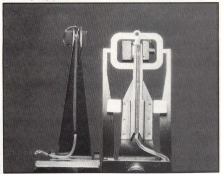
Comparison of Whitney (left) and Winchester (right) suspensions. Load beams are similar, but Whitney suspension has lighter, stiffer side rails. Result is more stable read/write platform with much lower flying height modulation in readback signal.
