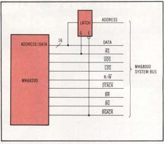
Fig 5 68200 connects to 68000 system bus via external address latch. All control signals can be connected directly.
