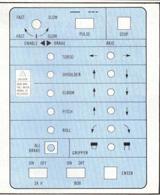
Fig 4 Handheld teach pendant programming aid. By manually controlling robot's motion with teach pendant, users can quickly and easily program robot for most pick and place tasks.
