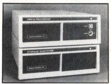
CMS16/UNX system combines the 68000 processor, MULTIBUS compatibility, and UNIX Version 7 OS in a single package. System uses a variety of software including C, Pascal, FORTRAN, BASIC, and COBOL. IEEE 796 system features the CMT-CPU 68000 16-bit microprocessor board based on the MC68000. Unit is available in OEM quantities, 30 days ARO. Cosmos Systems, Inc, 525 University Ave, Palo Alto, CA 94301. Circle 299
