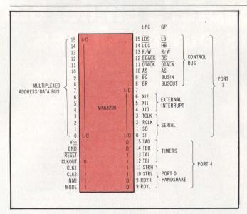
Fig 4  $\,$  68200 external bus logical pinout. 68200 has extensive repertoire of I/O functions.
