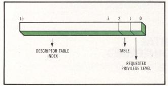
Fig 2 Selector part of virtual address. Selector specifies which table (and descriptor within table) will generate physical address. Privilege level is also indicated.
