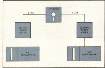
Compiled p-code Version IV UCSD p-System application is portable to any computer supporting p-System (including most 8- and 16-bit machines). When p-code is recorded on Universal Medium diskette, it becomes accessible to a wide range of computers by using adapter routines tailored to their disk formats.
