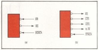
Fig 3 68000 bus arbitration lines. Only one device controls bus at one time (a). Asynchronous bus control lines require proper handshake (DTACK) from external devices (b).
