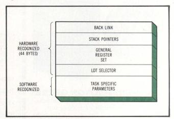
Fig 4 Task state segment used to support multitasking. Hardware and software specifics of each task are kept together, facilitating task operation.
