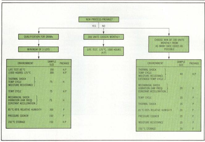
Fig 2 Tt's qualification program for 64k DRAMs. Devices are chosen at random. Numbers represent sample size per lot. "H" indicates hermetic package, "P" indicates plastic package.
