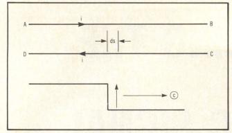
Fig 2 Transmission line equivalent circuit for digital logic signal analysis. Signal can be viewed as step propagating down each side of line.
