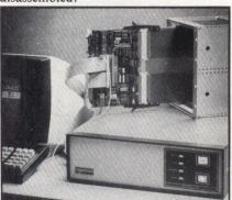
Debugging can be completed entirely within the UWS, or 64k bytes of the total RAM complement can be mapped into the system under development. An emulation cable and Footprint<sup>TM</sup> probe make all \$68000 pins available for connection of oscilloscope and logic analyzer probes, and provide full 8-MHz \$68000 hardware emulation.
