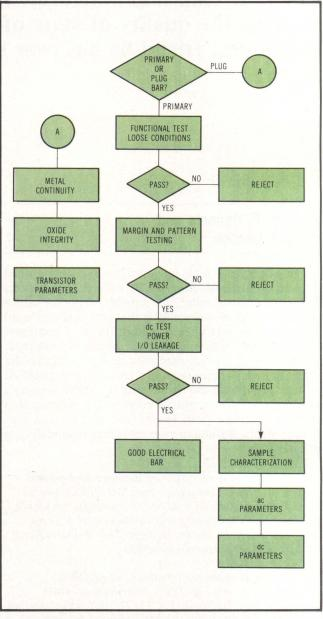
Fig 1 Block diagram of Multiprobe test program. Multiprobe begins testing chips before assembled for functionality, MOS parameters, and minimum and maximum dc parameters. "Primary" indicates 64k circuits, "plug" indicates test structures, and "bar" indicates a die.
