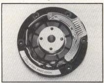
DB-3500-HD rotor/stator motor is set with 3 Hall-effect devices for commutation logic. It is compatible with DTL, RTL, TTL, or Mos circuits. Motor direct drives a disk load from standstill to 3600 rpm in 25 ms, and can develop 30 oz-in reserve torque for synchronism. No-load speed is 6300 rpm, with 54-oz-in stall torque. Rated voltage is 24 V. DB-3500-HD is 1.035" (2.629-cm) wide and weighs 14 oz (397 g). Clifton Precision, Litton Systems, Inc, Marple at Broadway, Clifton Heights, PA 19018.
