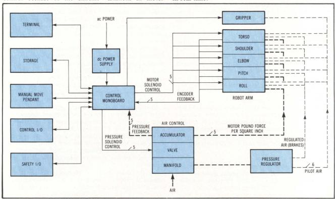
Fig 2 Robot system component block diagram. Monoboard oversees all facets of robot operation as well as provides means for 1/0 and system programming.
