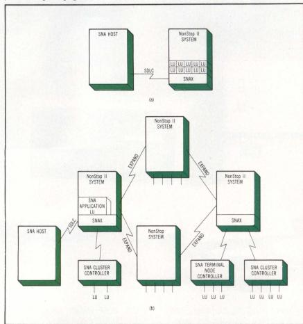
Viewed by host as cluster controller (a), several Tandem systems can support several SNA devices to reduce network management chores for host (b).
