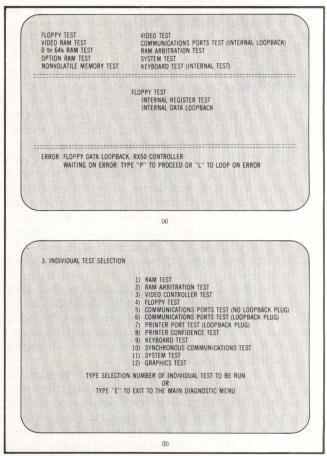
Fig 3 Extended diagnostics (a) are available on a diagnostic disk. If necessary, individual tests can be run separately from menu driven display (b).
