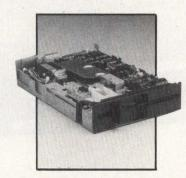
formerly occupied by a single Minifloppy. LSI electronics help to achieve the 10k MTBF POH and 30-min MTTR. Rotational speed is 300 rpm, with max inside track recording density of 5876 bpi for SA455 and 5922 bpi for SA465. Ambient temp range is 10 to
