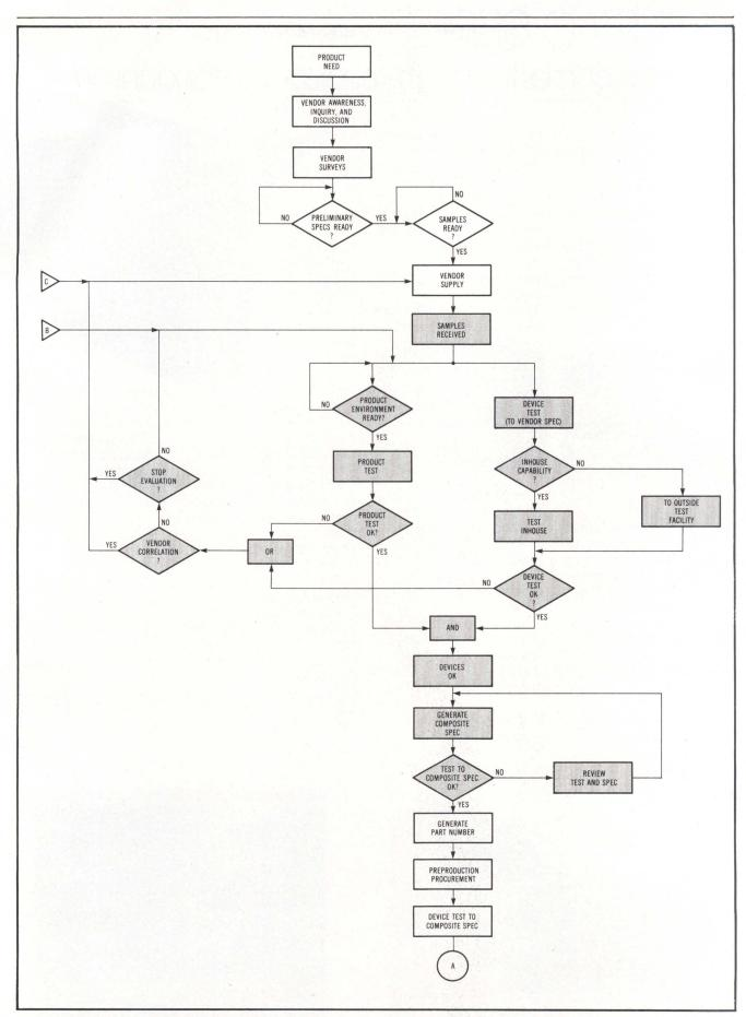
$Fig \ 3 \quad Prime's \ engineering \ qualification \ of \ 64k \ DRAMs. \ Program \ runs \ parallel \ tests \ on \ chips, \ both \ as \ individual \ devices \ and \ in \ product \ environment.$
