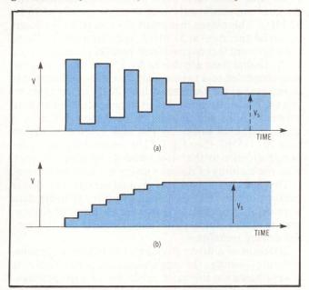
Fig 4 Digital pulse decay waveforms caused by impedance mismatch on signal lines. Vastly different waveforms associated with inductive ringing (a) and capacitive charging (b) result from differing amounts of signal reflection.
