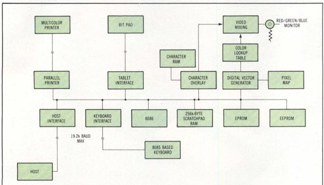
Workstation compresses graphics functions onto single board
