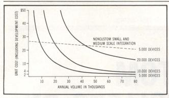
Fig 1 Cost/volume relationships for custom LSI of varying complexity. Software development costs are not included.
