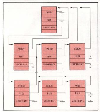
Fig 1 Relationship of typical system environment structures to each other. Each environment can point to three others via an internal table.
