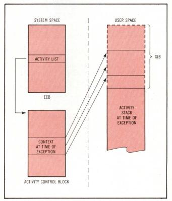
Fig 3 Exception data flow sequence. Once system determines that exception action is necessary and valid XVT is available, activity is initiated.
