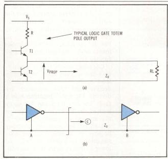
Fig 3 Logic gate action in typical digital application. Circuit of (a) shows that as signal edge travels from gate to gate (b) its amplitude is dependent on R and  $\mathbb{Z}_0$  only.
