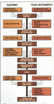
Teamwork is essential to successful logic array design. As shown, the TI design process divides responsibilities for maximum contribution by both parties and eliminates many manual, errorprone tasks.
