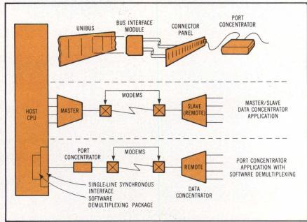
STATCON Series 21/11 bus driver remote configuration (top) is compared with traditional approaches. Neither traditional approach can simultaneously support both local and remote terminals.
