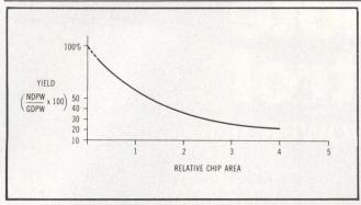
Fig 2 Net die per wafer (NDPW) is divided by gross die per wafer (GDPW), then multiplied by 100 to determine relationship between net die yield and die size.
