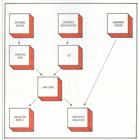
ICS within LANDS automatically reconciles hardware/software interface problems by generating all interrupt initialization and vector routines, linker commands, and library selections. It also performs consistency checks on requested setup and hardware configurations.
