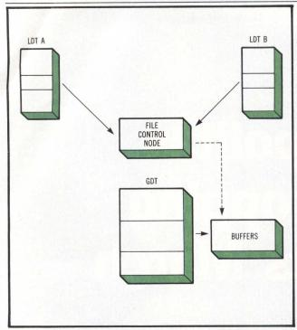
Fig 5 Task sharing of data structures. File control node allows tasks to access common file control blocks.
