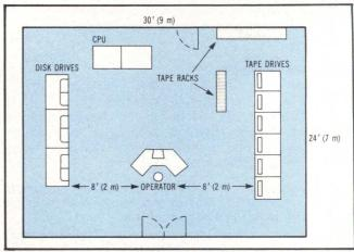
Fig 2 Physical layout of small DP center used in acoustic calculations and measurements
