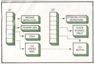
Fig 1 Descriptor based virtual addressing scheme uses descriptor tables for local and global segment access. Task specific and system-wide data structures can be referenced.
