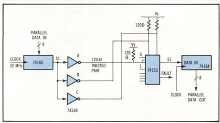
Fig 6 Triplicated serial data system using three twisted pairs. Both source and return lines must be connected close to integrated circuits.
