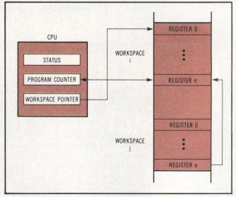
Fig 3 Memory to memory architecture employs multiple memory blocks as working register banks. Link vectors are stored in select workspace registers, eliminating need for stack.
