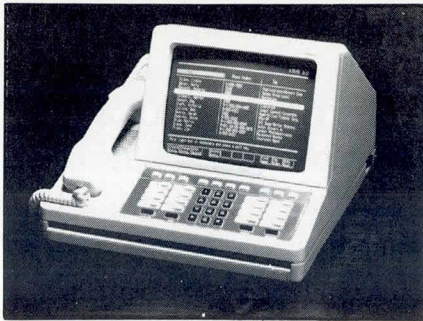
Cypress, Rolm's personal communication terminal, combines functions of a smart data terminal and a digital telephone to supply simultaneous voice and data communication.
