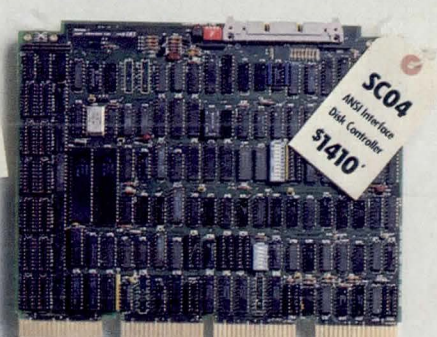
Handles up to eight ANSI 8" Winchester, emulates RK06/07 and RL01/02.
