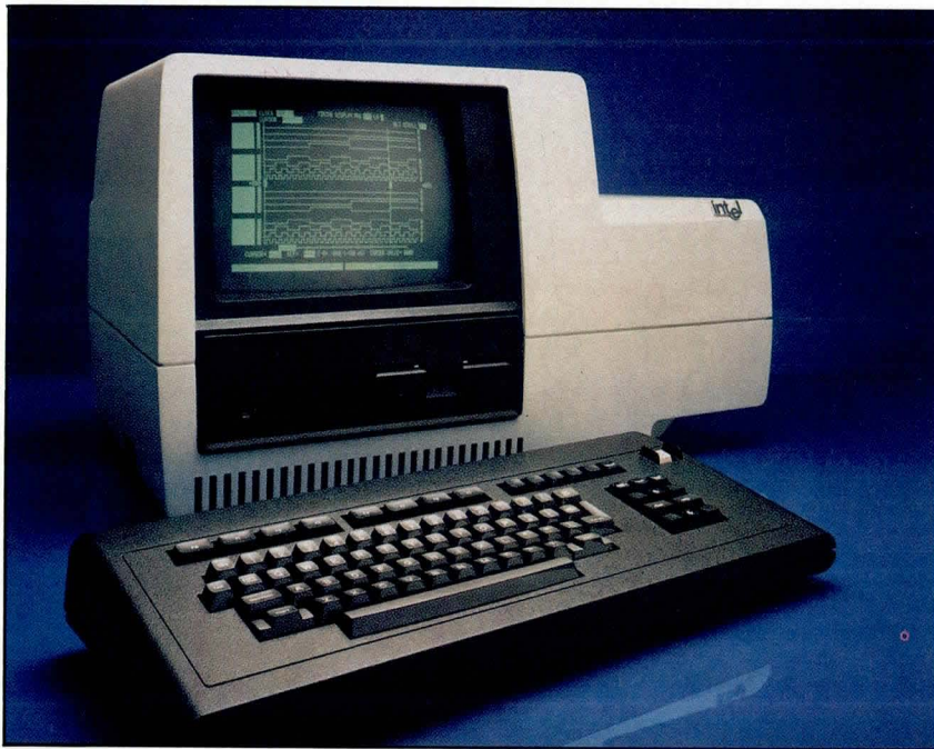
Combining hardware and software tools, the Intellec Series IV simplifies the design of products based on iAPX 86, 88, 186, 188, and 286 microprocessors.
