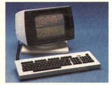
character generator; extensive alphanumeric and line drawing symbols; and compatibility with most standard, monochrome oriented, off-the-shelf software.
