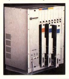
include local, remote, and mass memory. Local memory comprises the static RAM and/or erasable PROM (up to 128 Kbytes) that reside in the processor's eight memory sockets. Remote memory has the same capacity as local memory, but resides on the other processor boards in the system chassis. Mass memory consists of dynamic RAM on a dedicated memory board. Each processor board can directly access any portion of system memory unless it is prevented by interboard memory protect logic.
