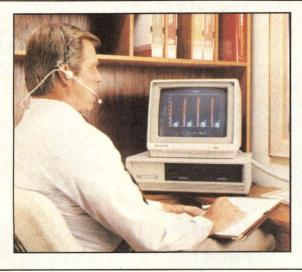
Speech Command, an option for TI's Professional Computer, adds voice 1/0 to the system's input and output repertoire. Recognizing connected streams of words, the unit has a 99-percent recognition rate.
