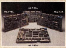
MLZ-90A single board microcomputer with nine byte-wide memory sockets for use with RAM or ROM (AM9511 and floppy disk drive controller optional).
