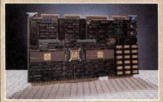
HK68™ powerful and versatile single board UNIXTM or CP/M-68KTM system with MC68000 CPU, MMU, quad channel DMA, four serial ports, 128K or 256K bytes of onboard RAM with parity (expandable to 1M byte on-board!), and two iSBX™ connectors for I/O expansion.
