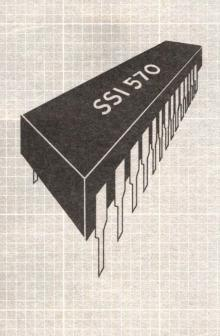
Silicon Systems' latest innovation in disk drive integration is the SSI 570. This creative design by Silicon Systems engineers integrates both the read and write data processing functions on one, 2-channel, monolithic IC. The circuit is designed for use with 8", 5-1/4", and 3-1/4" double-sided floppy disk drives.
