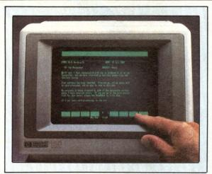
ating with IBM PCs to communicate with an IBM mainframe. Using a coaxial cable to an IBM 3274/76 communication controller and a modified communication board inside the PC, IBM PC users can retrieve data from the IBM mainframe using the touch-
