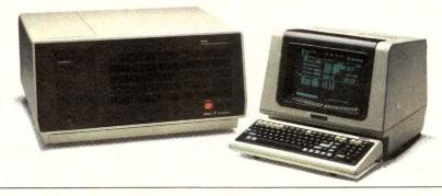
The Gould 9516S Microsystem Integration System supports **any** combination of 68000, 8086, 8088, Z8001, Z8002, 68B09E, 8085A and Z80A microprocessors. It includes a 1 megabyte thinline double-density, double-sided floppy disk drive. Its RS-232-C port lets you interface with any minicomputer for fast, effective software development.
