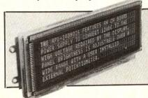
The 240-character APD-240M026 includes drive electronics and a dc-dc converter to develop necessary panel voltage. It provides six lines of 40 dot-matrix characters. Viewing characteristics include 30 ft-lamberts of brightness, neon-orange color, and 150-degree viewing angle. An external pot controls brightness. Basic price is \$450 in quantities of 100. Dale Electronics, Box 609, Columbus, NE 68601.
