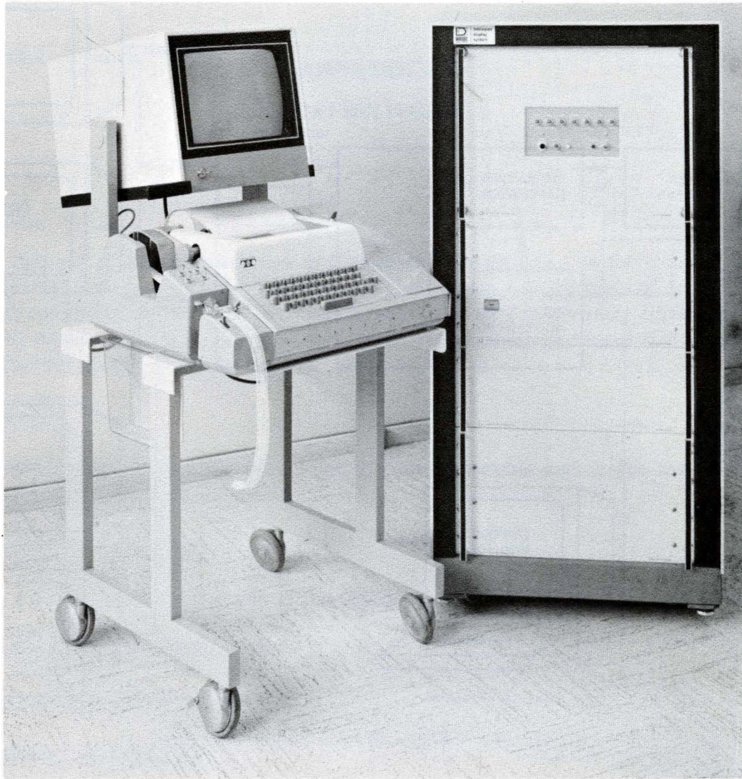
Figure 1-3. Data Disc TDS with Control Terminal
