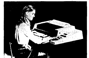
Dual Tape Cassette Transport Convenient magnetic tape medium can store 400,000 characters per cassette at 800 BPI, with a 120 inch/second search speed, and a variable record length of up to 1,000 characters.
