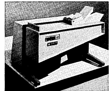
Card Reader Available in compact table-top or rack-mounted models, this unit reads 300 cards per minute and will handle 80- or 51-column cards.
