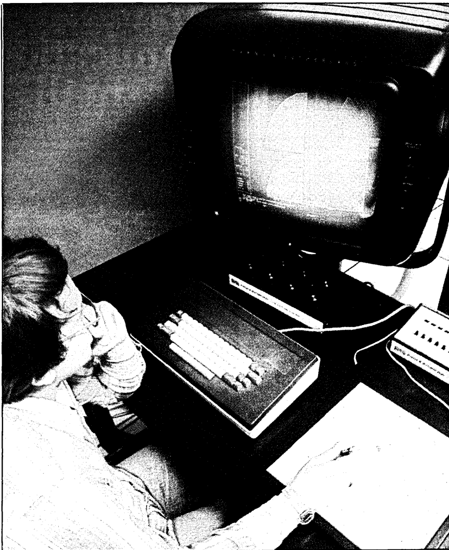
Fig. 4. The management and interpretation of the information produced actually becomes more of a problem as computers become faster. Los Alamos users frequently turn to interactive graphics, as illustrated here in the use of an Evans & Sutherland Picture System 2, and COM graphics, which is produced in movie and slide form.
