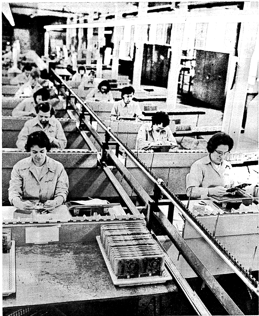
FLIP CHIP assembly line combines automated manufacturing steps with computer controlled checkout for lower cost, more reliable circuits.
