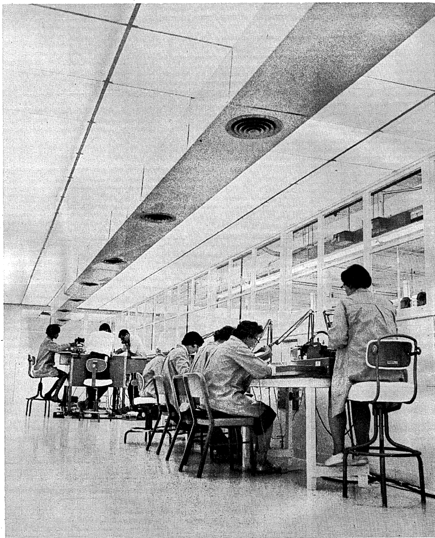
Substrate screening and semiconductor mounting operations are performed under clean room conditions.
