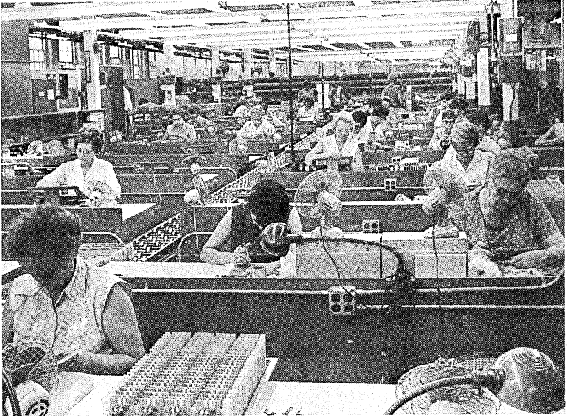
DEC Module assembly lines combine automated manufacturing steps with visual inspection and computer controlled testing.
