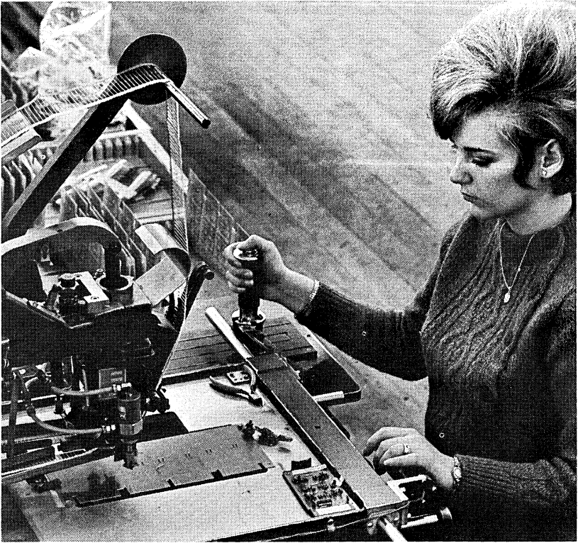
These pantograph-controlled insertion machines position and crimp pre-tested components onto four module boards at a time. A press will cut the modules apart after assembly is completed, minimizing handling up to that point.
