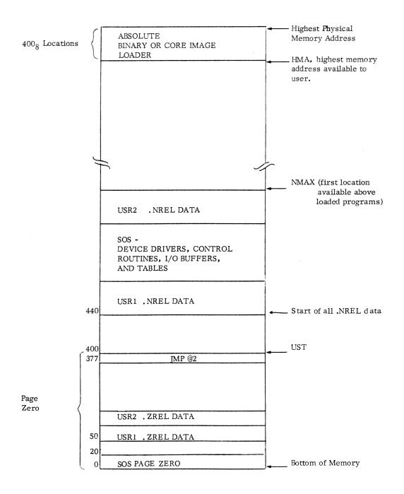
Figure 1-1. Loaded Program in Core
