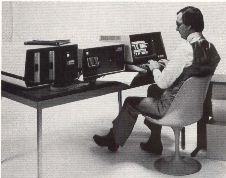
Microprocessor-system developer enters and edits programs on a Tektronix 8002 \mu P Lab. By changing a slave CPU card and an in-circuit emulation cable (visible in front of the development system's dual floppy-disk drives), the user can develop software and integrate it with hardware for both 8080- and 6800-based systems; future cards will accommodate the Z80 and other microprocessors.
