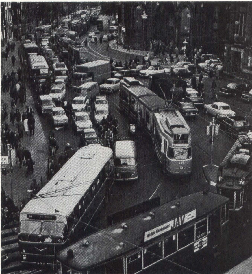
Subject to wide and almost unpredictable variations in traffic volume, sequential intersections like this one are ill-suited to control by inflexible, hardwired traffic systems. A microprocessor based system, however, can react readily to such intersections' constantly changing traffic conditions. (Courtesy Philips Telecommunication Review)
