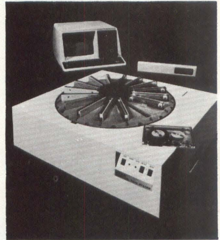
Carousel 5200 houses 16 3M-type tape cartridges in a removable pack and can load a cartridge into a read/write station in 2.7 sec.
