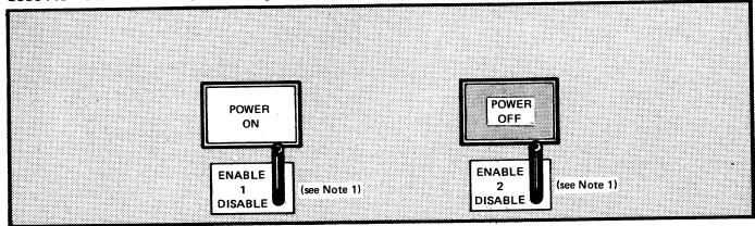
Power On: A momentary pushbutton that can be used to reverse the effect of the power off switch. If system power is on, and the power off switch is pressed to remove ac power from the drives, then pressing the power on switch will restore ac power to the 3333 and attached drives.
