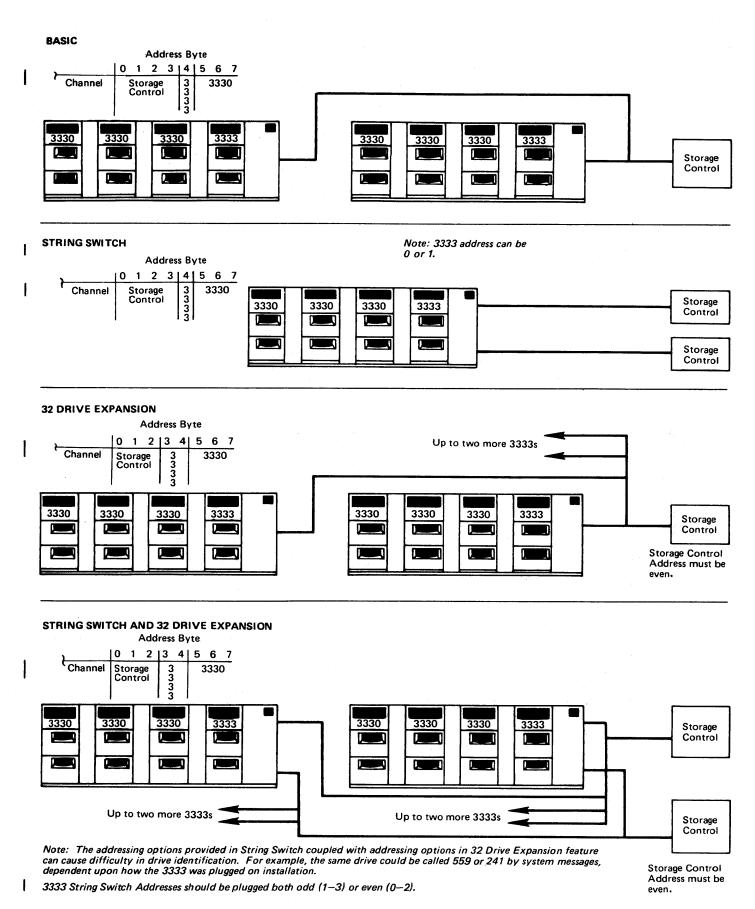
Figure 2. 3330 Series Feature Configurations
