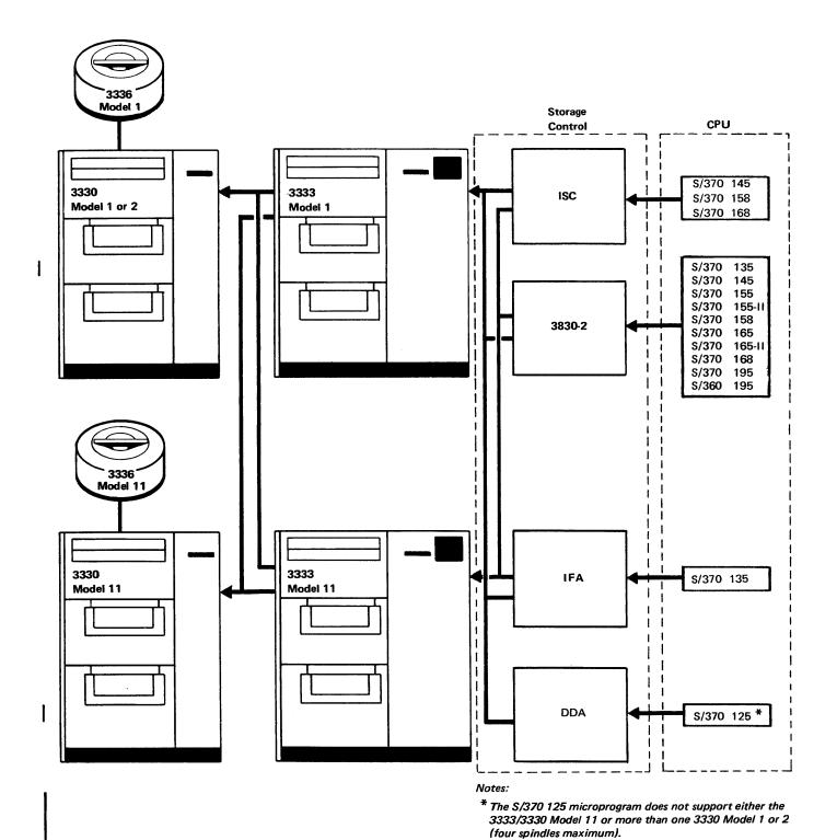
Figure 1. 3330 Series System Configurations
