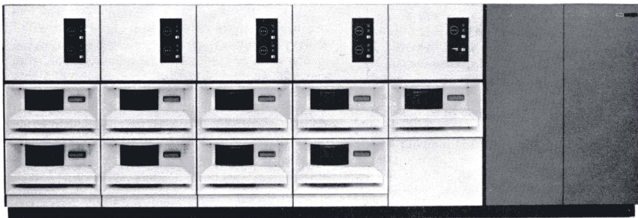
Figure 2. 2314 Direct Access Storage Facility
