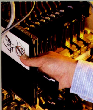
Dense packaging along with positive retention card-insertion features mean quicker upgrades with fewer failures.
