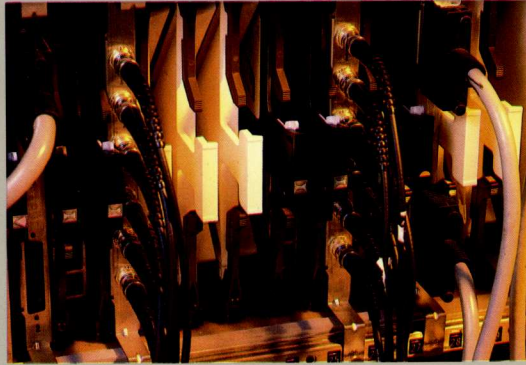
The processor's active tailgate design allows you to add I/O devices by simply plugging them directly into the appropriate I/O controller card.
