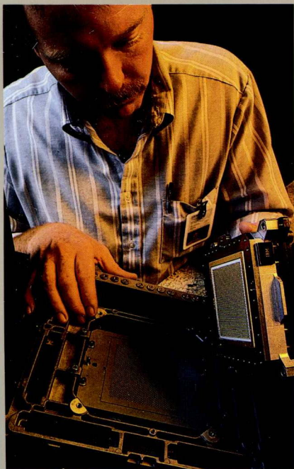
The 9370 Model 90 processor's single TCM mounts on a multilayer circuit board.
