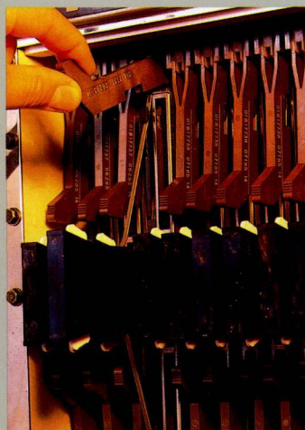
A card inserts easily into its slot. A retention spring on the card cover ensures that the card is positioned properly before the ZIF connector is actuated.
