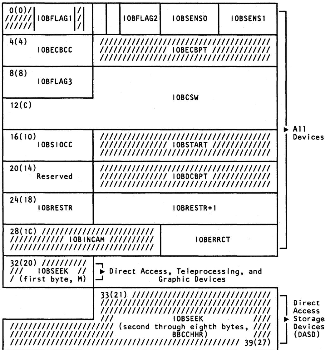
Figure 21. Input/Output Block (IOB) Format
