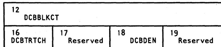
The system uses the contents of the block count (DCBBLKCT) field to write the block count in trailer labels when the data control block is closed or when the EOV macro instruction is issued. You must maintain the contents of this field yourself if the system is to have the correct block count. (Note: The I/O supervisor
