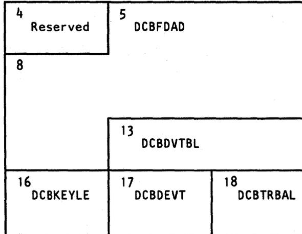
For output data sets, the system uses the contents of the full disk address (DCBFDAD) field, plus one, to write a file mark when the data control block is closed, provided the track balance (DCBTRBAL) field indicates that space is available. If DCBTRBAL is less than 8, the file mark is written on the next sequential track. You must maintain the contents of these two fields yourself if the system is to write a file mark. OPEN will initialize DCBDVTBL and DCBDEVT.
