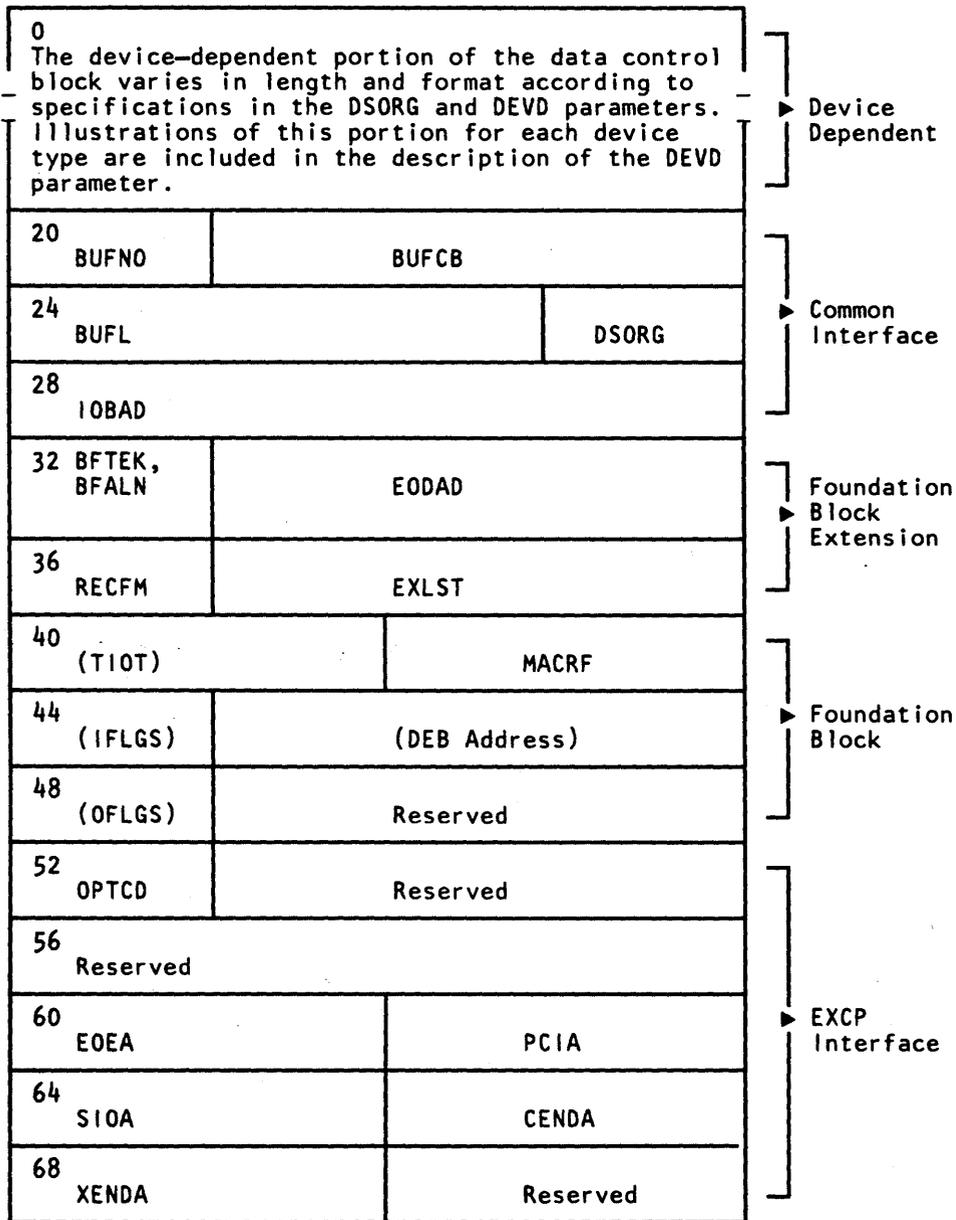
Figure 20. Data Control Block (DCB) Format for EXCP (After OPEN)
