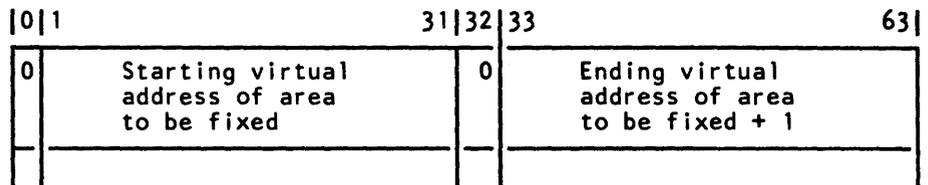
On return from your PGFX appendage to the EXCP processor (via the return address provided in register 14), register 10 must point to the first page-fix entry and register 11 must contain the number of page-fix entries in the work area. The EXCP processor then fixes the pages corresponding to the areas listed by the PGFX appendage. The pages remain fixed until the associated I/O request terminates.
