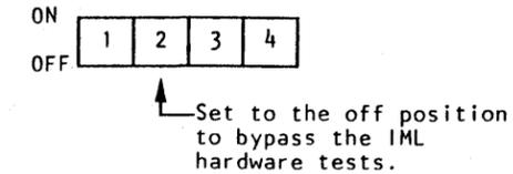
**Note:** All load control switches are set to the On position at the factory.
