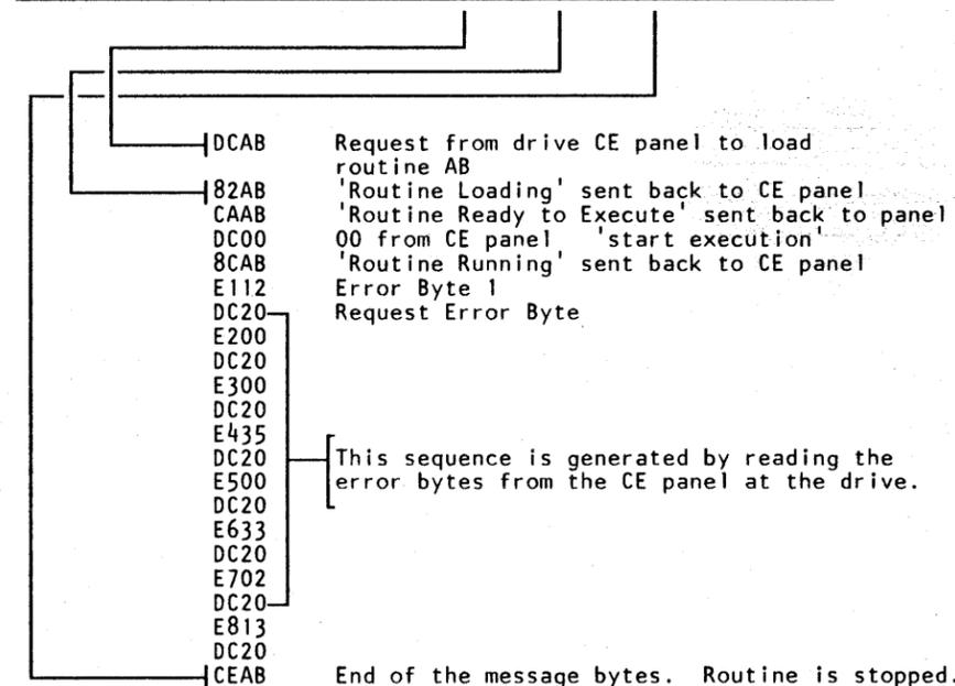
**Figure 1. Maintenance Connection Trace Table Sample**
