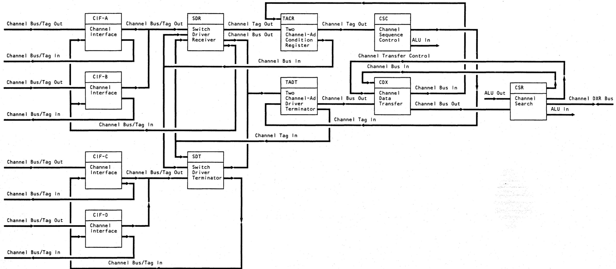
Channel Interface with Two Channel Switch—Pair, Additional Feature
