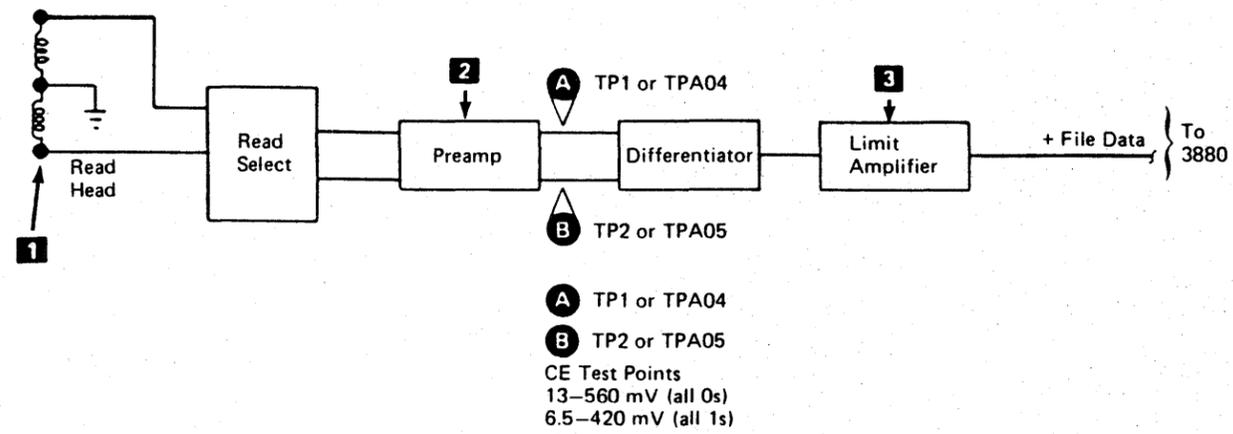
Full Track Differential Read Signal at CE Test Points
