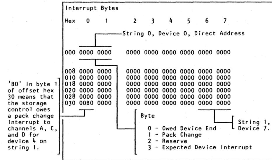
Figure 1. Interrupt Bytes Trace Table Sample
