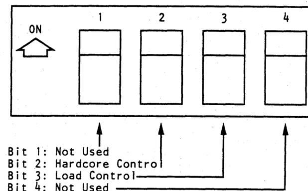
The label on the diskette shipped with the 3880 shows how the switches must be set for each storage director.
