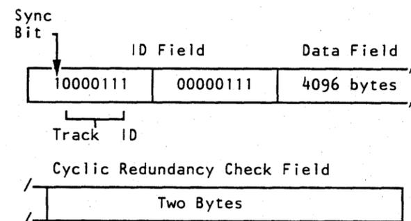
**Note:** The serial data read from a track is deserialized by the common overlay loader and controller in the common code.
