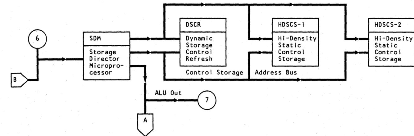
Data Transfer Between the Channel and the Port Adapter (CMCD Card)
