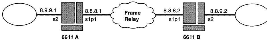
Figure 4-2. Sample Network for Routing TCP/IP Using Frame Relay over a Public or Private Network
