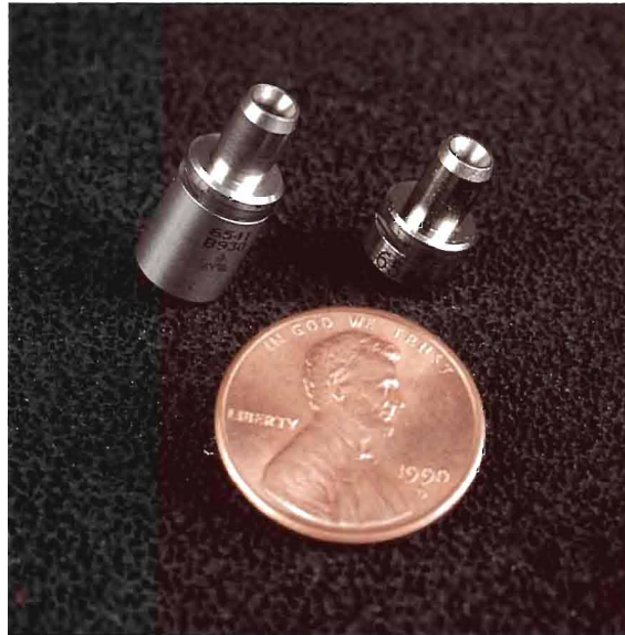
Figure 94. Laser (Left) and Detector (Right) Receptacles
