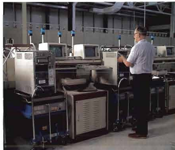
Figure 122. Test and Software Preload Station
