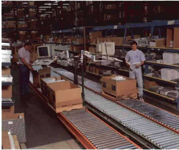
Figure 124. Bar Code Equipment in Use in the Packaging Process
