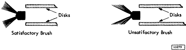
Figure 4-5. Disk Pack Brush Condition
