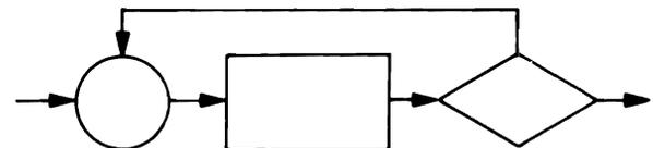
Figure 3. The DOUNTIL structure
