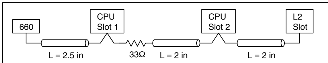
Figure 14. Data and Data Parity Path
