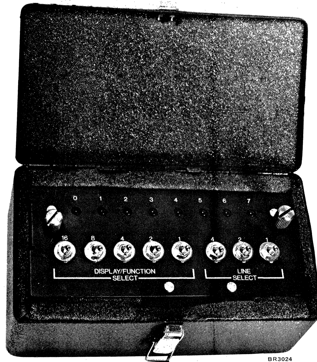
Communications panel in carrying case
