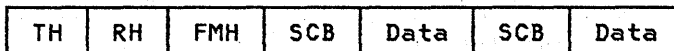
Figure 4-1. Examples of RU formats. The PIU is composed of the TH (transmission header), RH (request/response header), and RU (request/response unit). Although the use is not exclusive, path control (PC) uses the TH, transmission control (TC) and data flow control (DFC) use the RH, and session presentation services (SPS) and end users use the RU. The data formats are representative; not all formats are shown.
