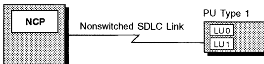
Figure 59. SDLC Devices Attached to Nonswitched Telecommunication Links
