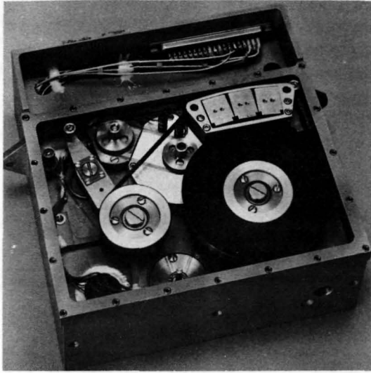
FIGURE 13-37.—A 10^7 bit-capacity spaceprobe recorder employing two motors and a plastic-belt differential drive (see text).
