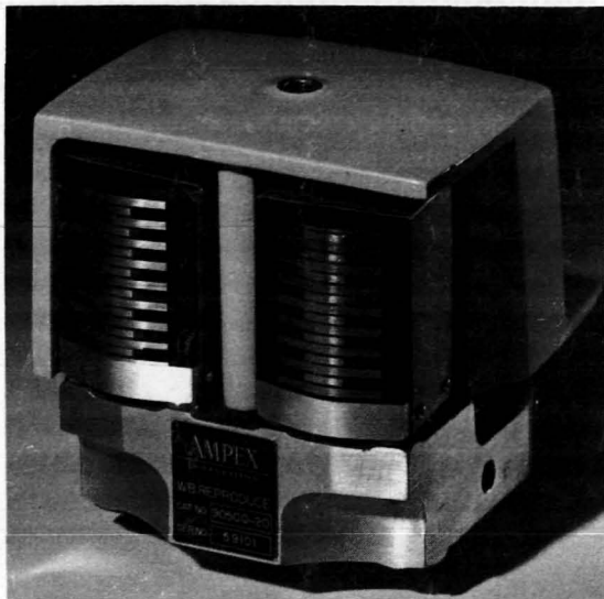
FIGURE 8-8.—Typical multitrack heads with relief between pole pieces.
