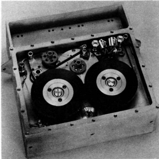
FIGURE 13-38.—The improved 10^7 bit-capacity spaceprobe recorder employing a single motor drive.
