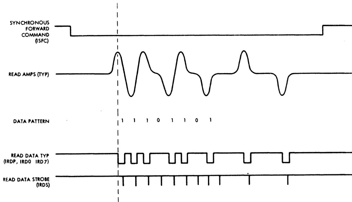
Figure 5. Typical Read Timing Diagram
