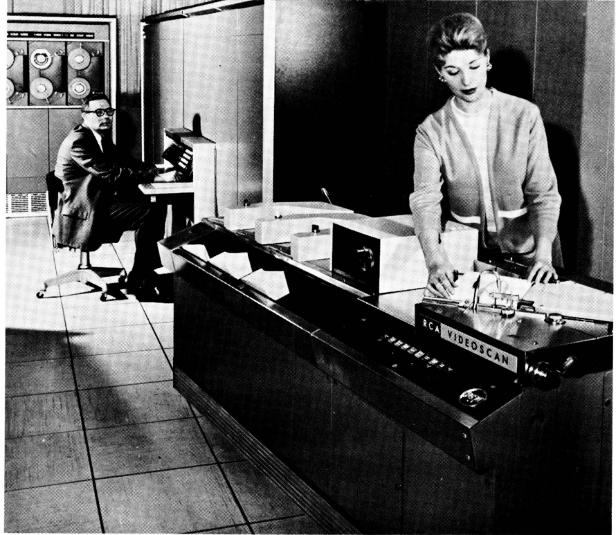
Fig. 4—A prototype VIDEOSCAN document reader which, utilizing the TV vidicon tube, allows high-speed reading of input documents—for example 90,000 utility bills, premium notices, and similar turnaround documents—directly into the RCA 301 computer, here shown in the background.
