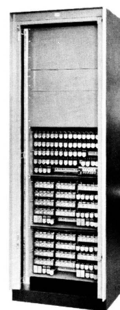
Fig. 5—A Model 6244 line concentrator with the door and cover panels removed. Model 6242 provides two output-trunk connections to two receivers, while Model 6244 provides four output-trunk connections to four receivers.
