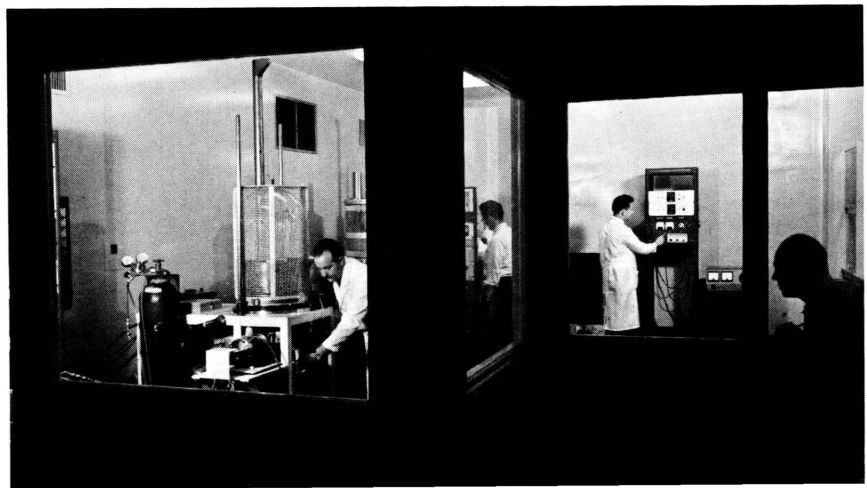
Fig. 10—White room and facilities for superconductive thin film fabrication.
