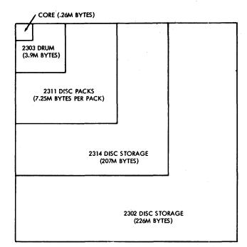
Figure 1—Relative capacity of various ADEPT direct-access storage media available in less than 0.2 seconds. The initial system that operates at SDC utilizes core, 2303 drum, 2311 and 2314 disc packs, and 2302 disc storage. The NMCSSC system utilizes 2314 disc storage in lieu of 2311 or 2302 discs. The architecture of the ADEPT executive is such that it permits any combination of the above types of disc storage in varying amounts
