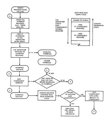
Figure 5—Block diagram of EXEX behavior and control
