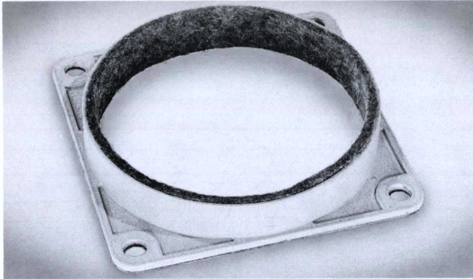
BE510 Bezel, for mounting camera on Tektronix 5" oscilloscopes. Dimensions—5 7/8" square; ring 7/8" deep, diameter 5 5/8" outside, 5 1/8" inside. Die-cast construction, wrinkle finish, felt lined. . . . . 4.50
