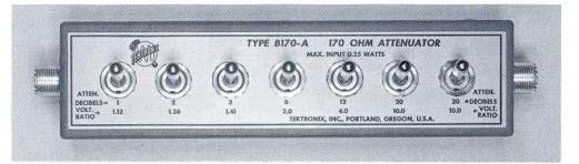
$170-\Omega$  pi-attenuator, uses 2% precision resistors, 1 to 64 db in 1 db steps, 0.25 watt.
