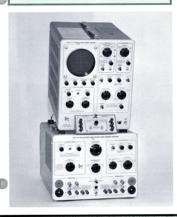
The Type 575 Transistor-Curve Tracer displays the dynamic characteristic curves of both NPN and PNP transistors on the screen of a 5-inch cathode-ray tube. Several different transistor characteristic curves may be displayed, including the collector family in the common-base and common-emitter configuration. In addition to the transistor characteristic curves, the Type 575 is used to display dynamic characteristics of a wide range of semi-conductor devices.
