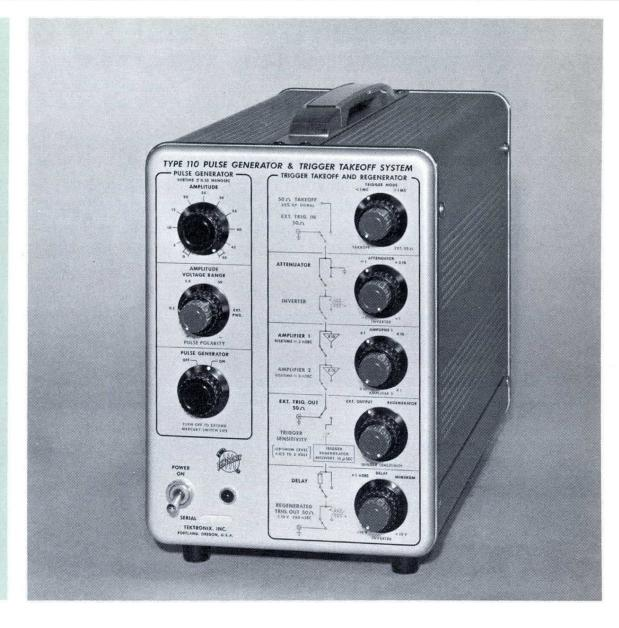
An externally applied trigger signal can also appear as an output after it has either been amplified, attenuated, or regenerated.
