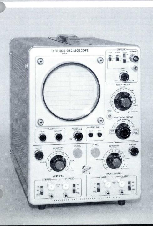
IDENTICAL VERTICAL & HORIZONTAL AMPLIFIERS DIFFERENTIAL INPUT AT ALL SENSITIVITIES **ELECTRONICALLY-REGULATED DC SUPPLIES** COMPACT CABINET OR RACK-MOUNT MODELS
