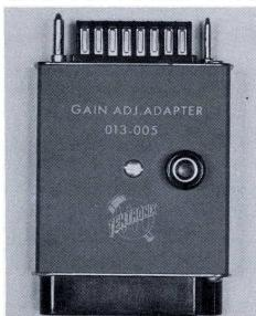
GAIN ADJUST ADAPTER—Permits an external calibrating signal to bypass the plug-in preamplifier, for calibrating the sensitivity of the main amplifier of Types 530, 540 and 550-Series Oscilloscopes.
