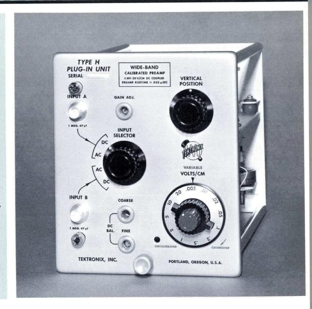
The Type H is a wide-band preamplifier with dc-coupling over its full sensitivity range. It provides a maximum sensitivity of 5 mv/cm, dc-coupled, in Types 530, 540, 550 and 580\* Oscilloscopes, with excellent transient-response characteristics.
