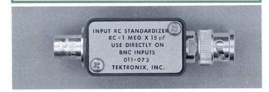
Five input time-constant standardizers are available for standardizing input capacitances of 12 pf, 15 pf, 20 pf, 24 pf, and 47 pf. Each standardizer has an approximate 1 megohm impedance and 2X voltage attenuation.
