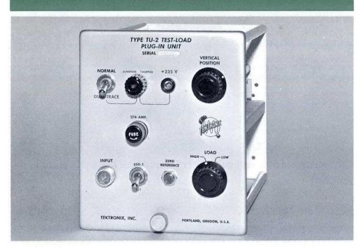
TYPE TU-2 TEST-LOAD PLUG-IN UNIT—The unit is used to check Tektronix Type 530, 540, 550-Series Oscilloscope power-supply regulation under high load and low load demands of A to Z plug-in units. It can also be used to check vertical amplifier balance, vertical amplifier gain, and dual-trace function of the oscilloscope.
