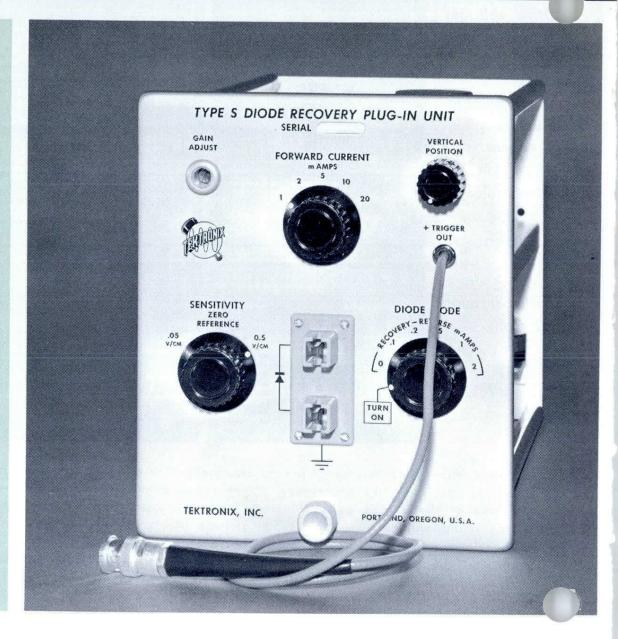
The Type S Unit enables you to display semiconductor-diode switching characteristics on your Tektronix Plug-In Oscilloscope. With Tektronix Type 540-Series, Type 550-Series, and Type 580-Series\* Oscilloscopes you can find:
