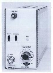
The 7A16A is a wideband plug-in amplifier for all 7000-Series mainframes. It features constant bandwidth over the deflection factor range of 5 mV/div to 5 V/div. Polarity of the display is selectable, as is bandwidth, which can be either FULL or limited to 20 MHz for low frequency applications.
