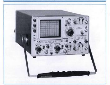
485 Oscilloscope—The 485 is a 350-MHz, 1-ns/div, 20.5-lb portable dual-trace oscilloscope. In addition to significantly advancing portable measurement capabilities, the 485 has many other new features. These features include selectable input impedance, trigger holdoff, external trigger display, alternate delayed sweep with trace separation control, vertical scale-factor indication, auto-focus, and B sweep intensity control.
