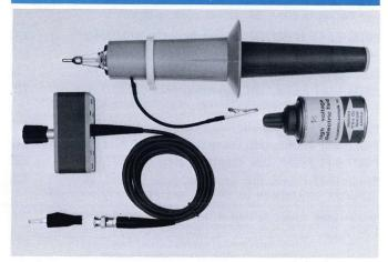
The P6015 provides 1000X attenuation for oscilloscope measurements up to 40-kV peak. Voltage or duty cycle derating is necessary for RF voltages at frequencies over 100 kHz, or in temperatures above 25°C.
