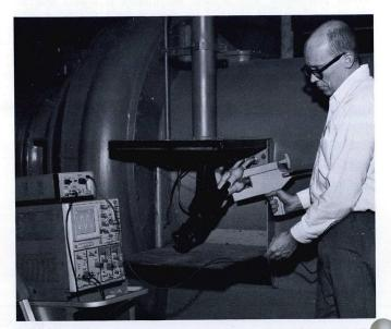
Typical application of the CT-5 clip-on high-current transforme P6042 DC current probe and 7000-Series Oscilloscope measuring the running current of a 1500 hp delta-connected induction motor.
