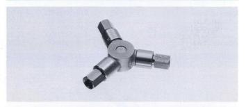
This coaxial tee is designed for use in broad-band,  $50-\Omega$ , systems where the mismatch introduced by ordinary "Tee" connectors is undesirable. Load isolation is nominally 6 dB while the voltage attenuation ratio is nominally 2X (input to either load arm, other load arm terminated in a standard  $50-\Omega$  termination). Maximum VSWR is 1.50 from DC to 12.00 GHz and 1.00 from 12.01 to 18.00 GHz 1.90 from 12.01 to 18.00 GHz.
