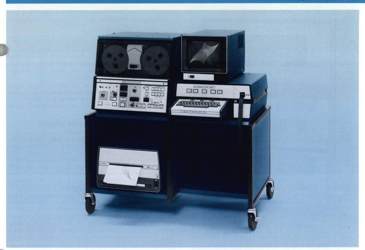
The 1781 Editor is an integral part of the TEKTRONIX N/C Editor System. The N/C Editor System consists of a 1781 Editor, a 1791 N/C Program Verifier, and a 4601 Hard Copy Unit, all housed in a mobile 207-1 Cart.
