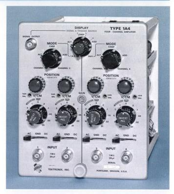
547, 549 and 556 Oscilloscopes. The front-panel output can also be cascaded with another channel, providing additional gain useful in many applications. Signal output amplitude is  $>\!0.5\,\text{V/cm}$  of display signal, unterminated at 1 kHz. Bandwidth is  $\leq\!20\,\text{Hz}$  to  $\geq\!10\,\text{MHz}$  (to approx 500 kHz with any channel operated in chopped mode). Approx 50- $\Omega$  output impedance.
