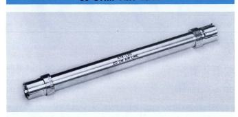
The 20-cm 50- $\Omega$  air line is useful as a time-delay device and as an absolute impedance in a time-domain reflectometer system. The characteristic impedance is 50  $\Omega$   $\pm$ 0.4%. Time delay is 0.6698 ns  $\pm$ 0.4%. Order 017-0084-00 \$18.75
