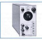
**5A19N Amplifier**—The 5A19N is a low-cost differential amplifier for the 5103N Oscilloscope System. Featuring low cost and simplicity of controls, it is ideal for monitor and systems applications.
