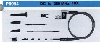
The P6054 is a miniature, fast-rise, 10X probe designed for use in conjunction with TEKTRONIX Oscilloscopes having a nominal input capacitance of 15 to 24 pF. The probe does not incorporate CRT READOUT/trace-identify functions.
