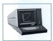
4013 Computer Display Terminal—One of the most exciting recent developments in computer technology has been the availability of a new programming technique called APL—A Programming Language. The TEKTRONIX 4013 Computer Display Terminal supports the full APL character
