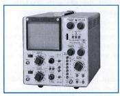
D66 Oscilloscope — The D66 provides 25 MHz bandwidth at 10 mV/cm. X10 gain expands the sensitivity to 1 mV/cm at 15 MHz bandwidth. Sweep rates extend from 2 s/cm to 100 ns/cm (to 20 ns/cm with X5 magnifier). An X-Y function on the D66 projects the TELEQUIPMENT product line
