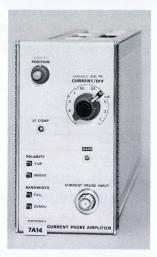
The 7A14 is an AC current probe amplifier for all 7000-Series mainframes. It provides constant bandwidth, dependent on the current probe and mainframe over the 1 mA/div to 1 A/div calibrated deflection factors (see bandwidth specifications). POLARITY is selectable, +UP or INVERT, as is BANDWIDTH, FULL or 20 MHz.
