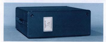
be TEKTRONIX 113 Delay Cable has a delay of 60 ns and characteristic impedance of  $50\,\Omega$ . In general it is used in those sampling applications where the vertical amplifier does not contain internal delay lines and the triggering of the sweep is external and signal delay is required.
