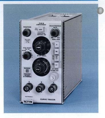
A front panel button switches the base/gate step generated output from current steps of the same polarity as the collector/drain sweep for checking transistors, to voltage steps of the opposite polarity of the collector/drain sweep for checking FETS in the depletion region. This button also internally switches the test fixture leads so that one test socket can be used to test both transistors and FETs.
