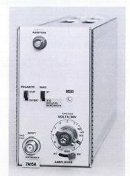
The 7A15A and 7A15AN are wideband plug-in amplifiers for all 7000-Series mainframes. They feature constant bandwidth over all the deflection factor settings. The two vertical mainframe channels allow the 7A15A/AN to be used alone, or with another vertical unit for dual-trace operation. Polarity of the display is
