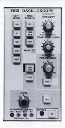
The TEKTRONIX 7613 Storage Oscilloscope offers Variable Persistence operation with a stored writing speed of 5 div/ $\mu$ s or conventional (nonstorage) operation. Stored traces can be viewed up to 60 minutes on a display area of 8 x 10 div (0.9 cm/div). The 7613 CRT is extremely burn resistant and doesn't require any special operating precautions.
