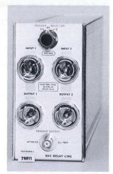
The 7M11 is a passive dual DELAY LINE unit for use with the 7000-Series sampling system. In low-repetition rate applications, requiring the sequential mode of operation, the 7M11 provides the trigger source and signal delay necessary to view the triggering event.
