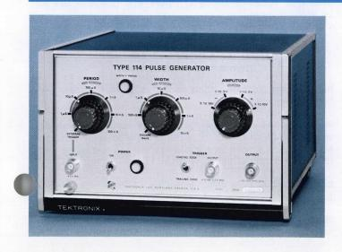
PULSES OR SYMMETRICAL SQUAREWAVES 10-ns risetime and falltime variable pulse period, width, and amplitude  $\pm$  10 V into 50  $\Omega$  short-proof output
