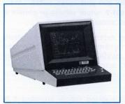
4010 Computer Display Terminal—The 4010 is the first low-cost large-screen terminal able to support alphanumeric and complex graphics. Equally adaptable to business, scientific, and academic environments, the 4010 is capable of portraying 2500 characters in alphanumerics, or complex graphics.
