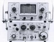
1401A-1 Portable Spectrum Analyzer shown with a 324P7 Oscilloscope
