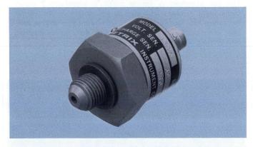
The Pressure Transducer is designed for use at engine speeds up to 6000 RPM, providing thread temperature is limited to 150° C. Engine speed must be derated to 1500 RPM when using the cooling adapter and to 1000 RPM when a 5-inch to 10-inch coupling pipe is used. The piezoelectric Pressure Transducer, when used with the charge amplifier of the Type 3A74 Engine Analyzer Amplifier and the included 50-ft low-noise cable, has the following characteristics.
