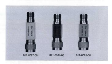
Attenuators are all supplied with Type N fittings. See accessory section for adapters for other series. Frequency range is DC to 12.4 GHz. Power rating is 2 W average, 300-W peak. Impedance is 50  $\Omega$ .
