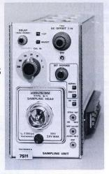
The 7S11 is a single-channel sampling unit for use in all 7000-Series mainframes. The input configuration employs the sampling "Plug-In Head" concept for maximum application range. The heads, which mount in the 7S11, cover a bandwidth from 350 MHz to 14 GHz. (See sampling head descriptions.)
