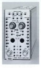
The high density of controls on a 2 5/8 inch by 5 inch front panel was made possible, and very usable, by the development and use of lighted push buttons for all except continuously variable functions. The switches conserve space both in front and behind the panel, provide faster operation (direct steps to any position) and easy readability by backlighting.
