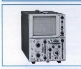
D83 Oscilloscope — A bandwidth of 50 MHz at 5 mV/div and the concept of plug-in selectability are the main features of this oscilloscope. The plug-ins include a differential amplifier, a dual-trace amplifier and a Dual Time Base. The CRT in the D83 is from the field-proven 7000-Series
