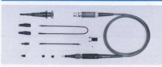
The P6052 is a passive dual-attenuation probe designed for TEKTRONIX low-frequency oscilloscopes that feature CRT READ-OUT and trace-identification functions. A sliding collar on the barrel of the probe selects 1X or 10X attenuation; a push button actuates the trace-identify function. A coding ring on the probe BNC output connector couples the control signals to the mainframe. The P6052 can be compensated for use with instruments having a nominal input capacitance of 15 to 55 pF.
