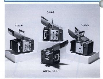
The C-53, C-58 and C-59 Cameras are the latest members of the C-50 Series Cameras. They are designed primarily for the 7000-Series Oscilloscopes, however, they may be used with most other full-size oscilloscopes and display units.
