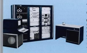
The S-3200 Series places equal emphasis on logic function testing, DC (parametric) testing and dynamic testing. System program and control is provided by the DEC PDP-11 Controller with a disc file being used for test pattern storage. Test programs and data may be stored on disc or on magnetic tape.
