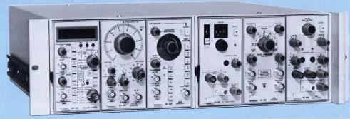
With a TM 503 and 604 Monitor or 603 Storage Monitor. Either monitor available with internal time base or may be swept with the RG 501 plug-in module.
