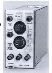
The 7CT1N Curve Tracer is a plug-in unit for use in TEKTRONIX 7000-Series Oscilloscope Systems. Characteristic curves of small-signal semiconductor devices to power levels up to 0.5 watt can be displayed. The 7CT1N operates in either vertical compartment. Horizontal deflection is achieved through a front panel source which drives the external input of either a vertical or horizontal plug-in unit installed in the mainframe's horizontal compartment.
