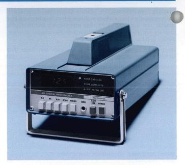
A silicon photodiode and a computer-designed glass filter are used to provide flat spectral response from 450 to 1000 nanometers within  $\pm 5\%$ . The response is typically down to 50% at 400 and 1060 nanometers.
