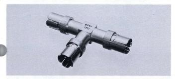
This coaxial tee has a 16.67-ohm resistor in each leg, connected so that the tee looks like 50 ohm if two legs are terminated in 50 ohm. It is designed for use in broad-band 50- $\Omega$  systems where the mismatch introduced by ordinary "Tee" connectors is undesirable. It is especially useful in a time-domain reflectometer set-up where test line, pulser, and oscilloscope must be coupled with a minimum of reflection-producing discontinuities.
