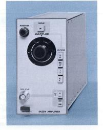
The 5A23N is a general-purpose amplifier for the 5103N Oscilloscope System. Featuring low cost and simplicity of controls, it is ideal for monitor and systems applications. It operates in the left or middle plug-in compartment of the 5103N mainframe for Y-T displays, or in the right compartment for X-Y displays.
