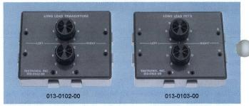
Designed to accept untrimmed bipolar or single FET's or transistors.
