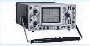
**475 and 465 Oscilloscopes**—The exceptionally low cost of the 465 with 100 MHz at 5 mV/div and the 475 with 200 MHz at 2 mV/div represents a price/performance breakthrough for portables and insures top value for the future.
