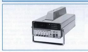
The TEKTRONIX J16 is a portable digital photometer/radiometer designed for use in the laboratory, or in the field. Illuminance, irradiance, and luminance measurements can be accurately made by selecting the appropriate probe. A choice of five probes is available. Each uses a silicon photodiode which has excellent long-term stability and reliability. Easy-to-read 2½-digit LED readout reduces measurement error, particularly in low ambient light conditions.
