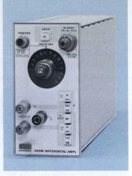
The 5A19N is a low cost differential amplifier featuring variable DC offset and simplicity of controls. It is ideal for monitor and systems applications and operates in the left or middle plug-in compartment of the 5103N mainframe for Y-T displays, or in the right compartment for X-Y displays.
