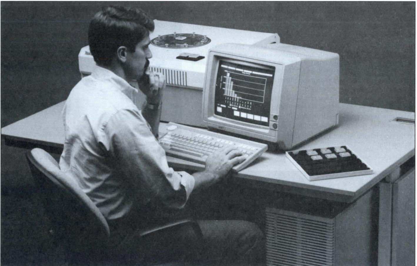
The DAS 9200 personal verification system supports application-specific IC (ASIC) functional verification, analysis, and debugging.
