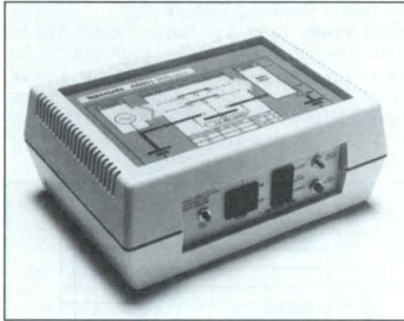
the power to the instrument is interrupted, a protective ground is reestablished, and an audible alarm is sounded. The A6901 also verifies the existence of a functional ground in the power source.
