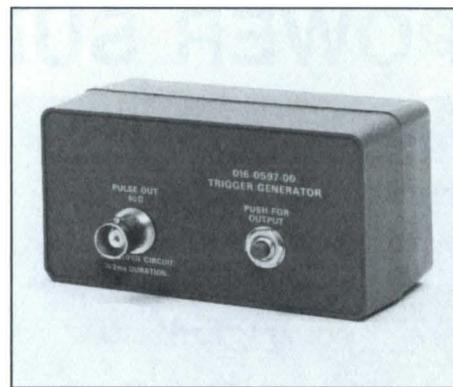
The Manual (one-shot) Trigger Generator is used for manually initiating a pulse or a complete train of events with instruments that do not have a manual trigger button or where a remote-operation capability is desired, such as with some oscilloscopes and the PG 501.
