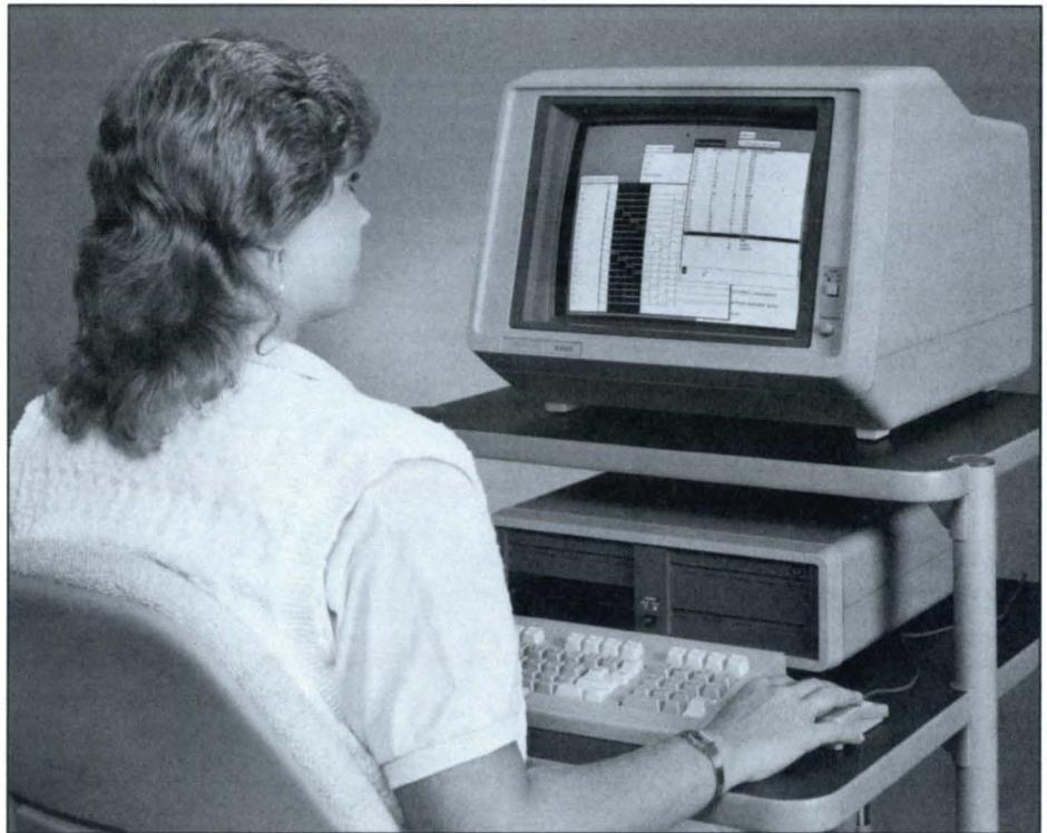
puter. The MicroVAX II is configured with 3M bytes of memory, a 31M byte hard disk, 95MB cartridge tape, and GPIB and Ethernet interfaces.
