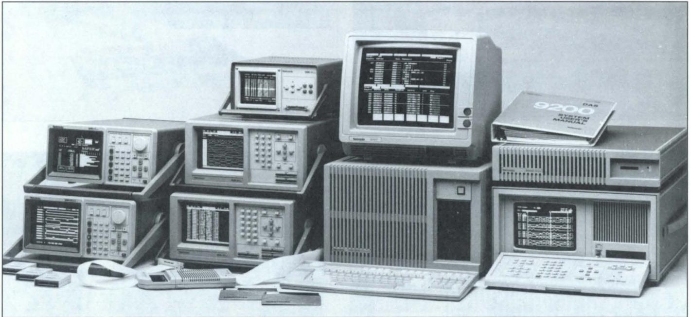
The Tektronix Logic Analyzer family includes the DAS 9200, DAS 9100, 1240/1241, 1220, 1225, and the 300 Series Logic Analyzers (not shown).
