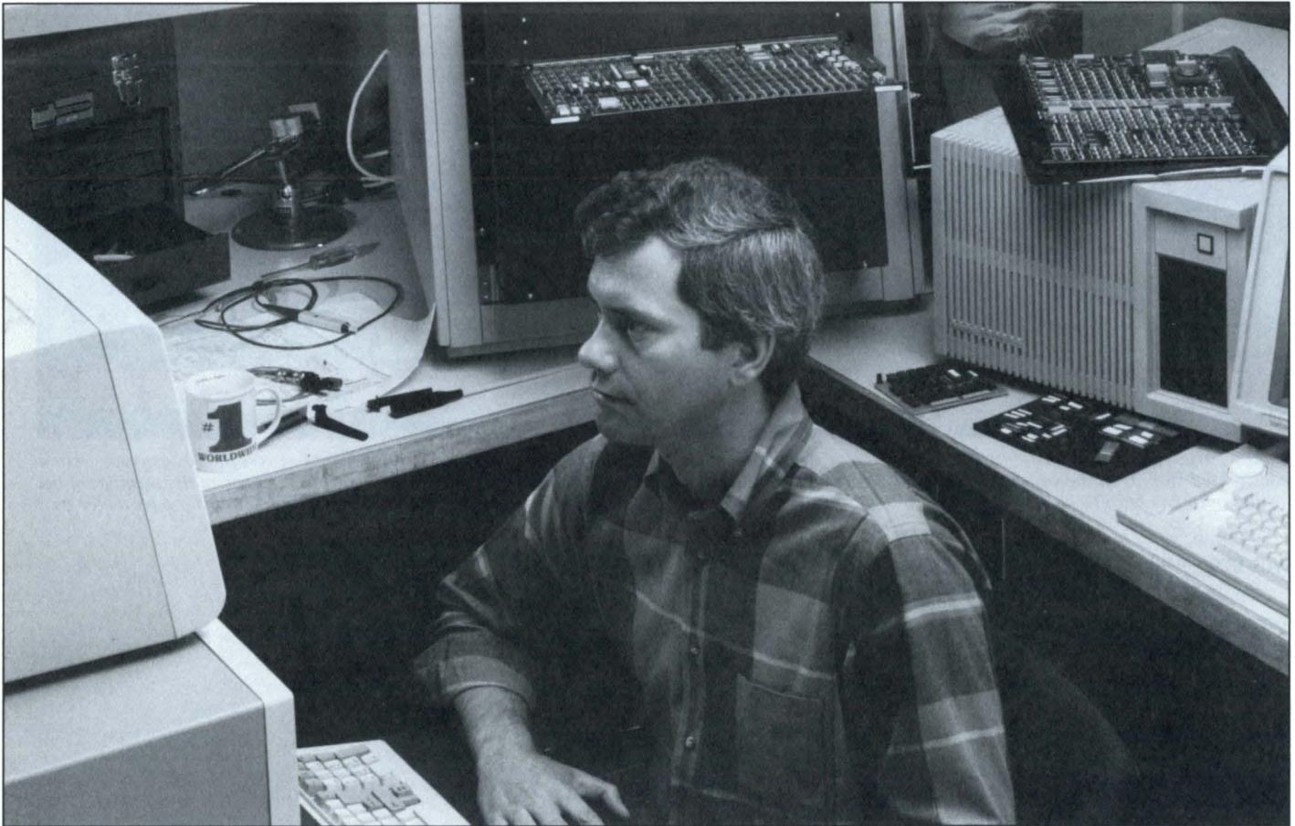
*Operable as a standalone device or under the control of a host (such as a PC), the DAS 9200 can move from engineering to manufacturing with no loss of functionality.*
