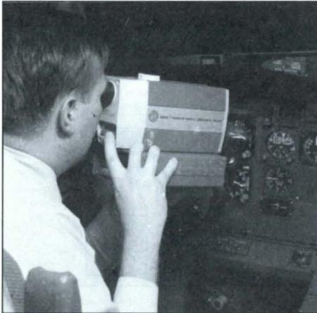
Measuring Luminance with the Tektronix J16/J6523.
