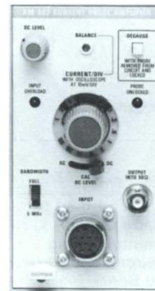
The AM 503 operates in any one of the TM 500 power modules and is connected to the A6302 or A6303 probes through a multipin connector.
