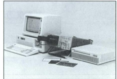
*DCS01 Digitizing Camera System captures repetitive waveforms from analog scopes and transients according to a scope's CRT writing speed (350 MHz for 2467).*
