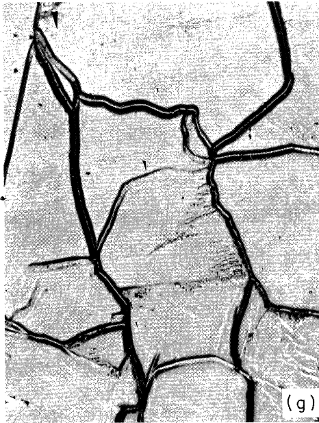
Fig. 6-30. (continued) Etch patterns on silicon. (From ASTM Method F47-64T. 20 ) (e) Twin boundary (200X); (f) twin lamella (200X); (g) grain boundaries (200X); (h) polycrystallinity — macro scale (3.2X).
