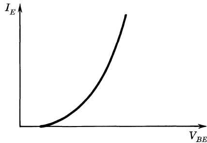
Fig. 23.7. Input diode characteristic curve.
