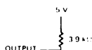
LOAD CIRCUIT FOR EACH OUTPUT NOT BEING PROGRAMMED OR FOR PROGRAM VERIFICATION FIGURE 1
