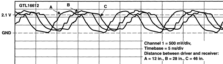
Figure 16. GTL16612 Signal Integrity at the Receiver Input Using Different-Length Cables
