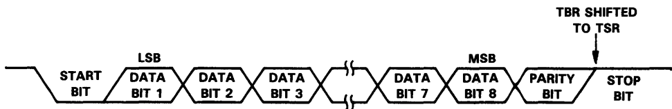
Figure 3-32. Asynchronous Transmission of Eight Bits Plus Parity
