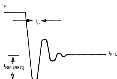
Figure 9 - Reverse Recovery Time of a Rectifier
