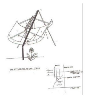
An additional mechanismallows the operator to vary the angle of the collector with respect to its axis of rotation, thus accommodating seasonal changes in the angle of incidence of the sunlight (angle at which sunlight strikes the collector). The position of the turning axis can be adjusted so that the collector remains as perpendicular as possible to the sun as it rotates through out the day.
