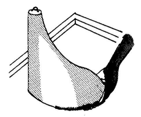
FIGURE 8. SEALING CRACKS WITH CLAY.
