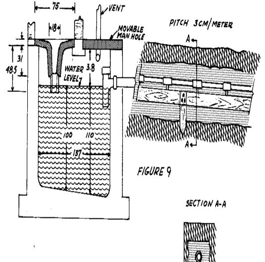
tank. This forms a water seal, which keeps bad odors from rising into the privy shelter.
