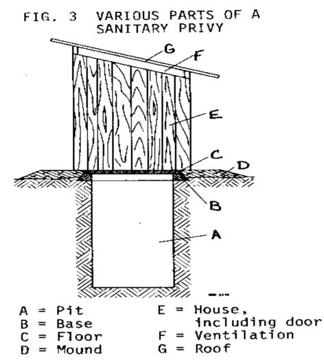
otherwise might enter and destroy the pit. It should be built up to the level of the floor and be very well tamped. It should extend 50cm (20") beyond the base on all sides. The mound may be built much higher than the ground in areas where
