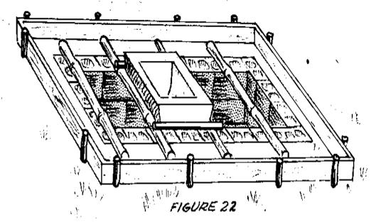
in half across the pit as a base for the slab. Place the bowl between two of the bamboo pieces with a piece of wood under the front and back; nail these to the bamboo. After the bowl is positioned in this way, pour water into it to be sure it
