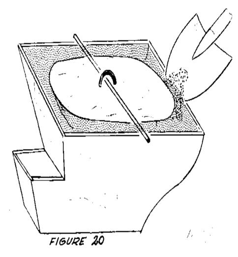
cement around the mold with a stick and pack it well to get rid of air spaces.
