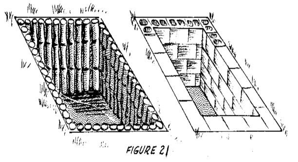
Place boards around the outside of the pit 15cm (6") from the edge of the pit to form the perimeter of the slab (see Figure 22). Place large pieces of bamboo split
