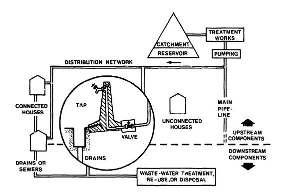
FIGURE 1: COMPONENTS OF STANDPOST WATER SUPPLY SYSTEM
