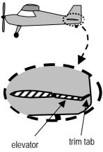
An aeroplane is made to point up or down by raising or lowering the elevators at the back of the aircraft. Along the rear edge of the elevators are trim tabs, which are used to keep the elevators in the correct position for the particular load that the aircraft is carrying. The trim tabs are very small, but if they are not set correctly, the pilot must fight against them all the time to keep the aircraft at the correct height.
