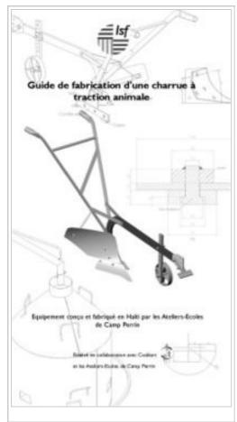
Technical sheet Soil type: any type of soil but ideal for heavy soil medium, which is not too stony Traction: a pair of oxen Stability: longitudinal Coulter: duck beak-type, width 8 " Versoir: cylindrical type Use: for small sized holdings (<4 ha) or in addition to more heavy machinery in larger establishments Features:: locally produced, low manufacturing cost, simple manufacturing techniques.
