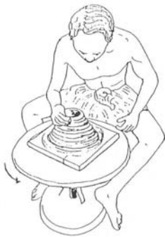
8. Pulling inwards and upwards, raise the outer part of the clay.
