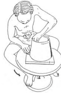
19. Using a wooden "rib", straighten the wall and remove excess clay.
