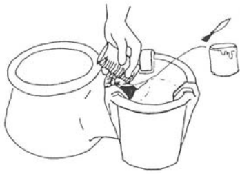
54. Score and slip the rim between the two potrests closest to the firebox.
