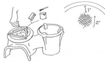
80. Place the triangle template so that one point is on the side of the firebox. Mark inside underneath the points. One inch below the rim, score and slip a 2" diameter area.
