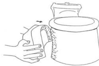
74. Place the door and mould against the firebox, aligning the mould with the door opening.
