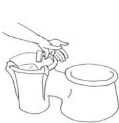
61. Place the shield on the rim, and press to make a strong joint.
