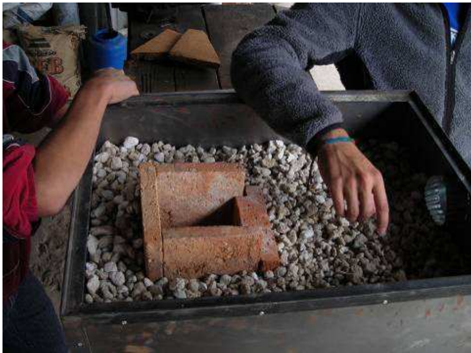
A small chamber to allow space for the smoke to flow out is made in front of the chimney using baldosas.
