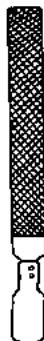
Rasp, needs to be replaced every 2 months in normal use (used to trim the foot)
