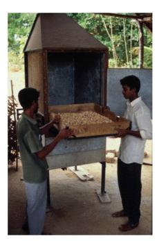
Figure 6: The Practical Action Tray Dryer in Sri Lanka ©Practical
